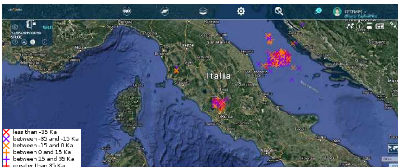
Figure 6.4.1: location and the intensity (expressed as positive or negative amperage) of the lightning strikes observed on May 12, 2019 from 02:00 to 05:00 UTC
