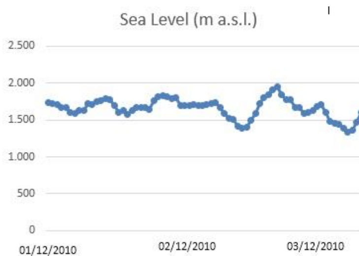
Figure 4.1.3: sea level measured in the Ploce station (data from HHI – Hydrographic Institute of the Republic of Croatia)
