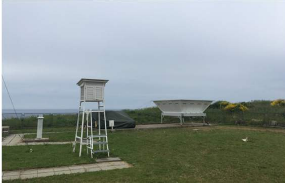
Figure 14 The wind profiler installed at GMP Dubrovnik (on the right side of photo).
