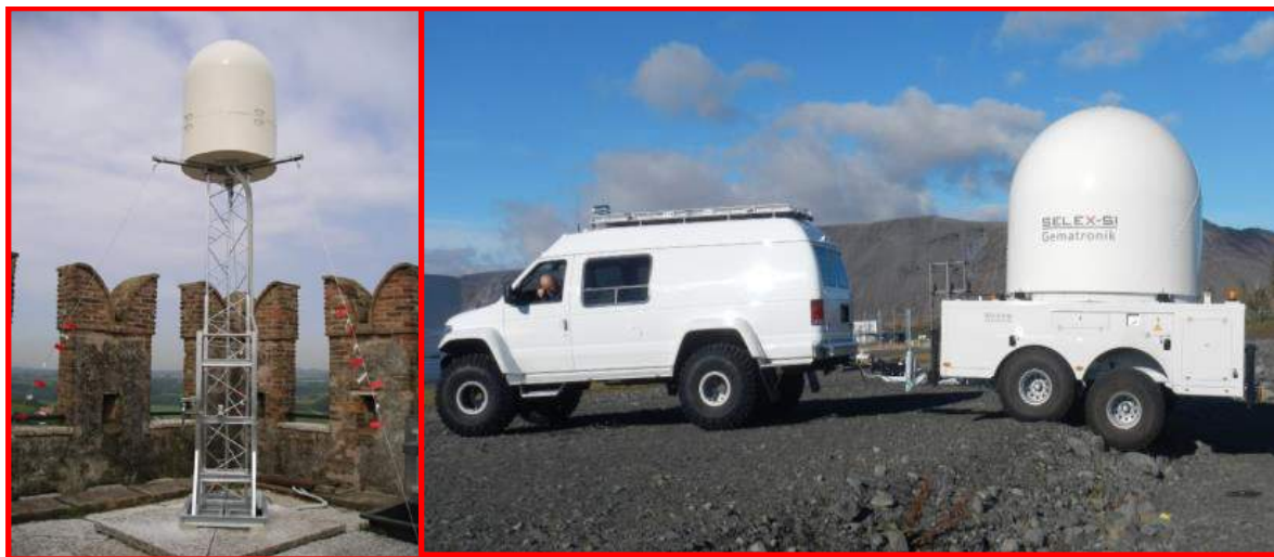
Figure 3.8 X-band radar installed on fixed (left) and mobile platform (right panel)
