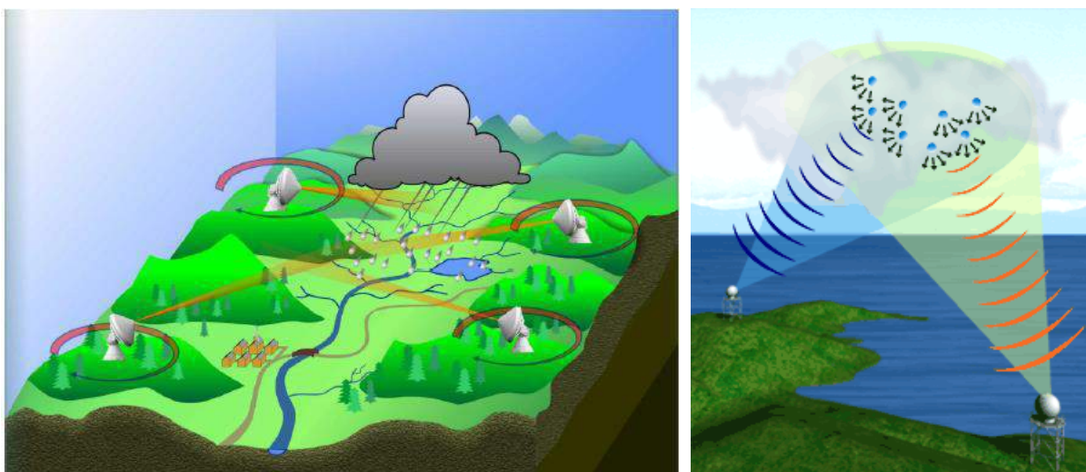
Figure 4.1 Conceptual images illustrating a network of radars operated as a single instrument
