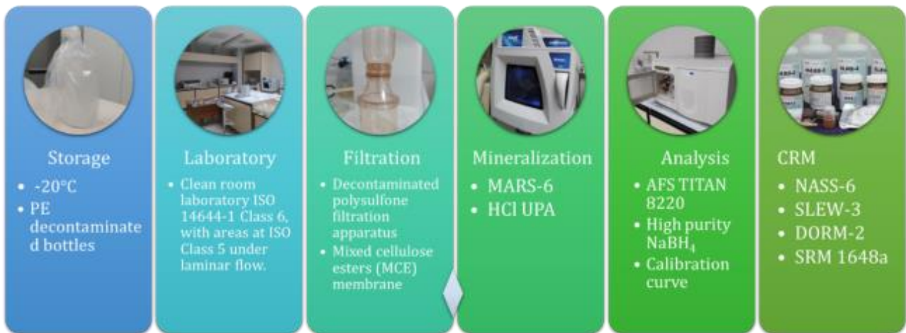
Figure 44. Analytical procedure for metals determination.
