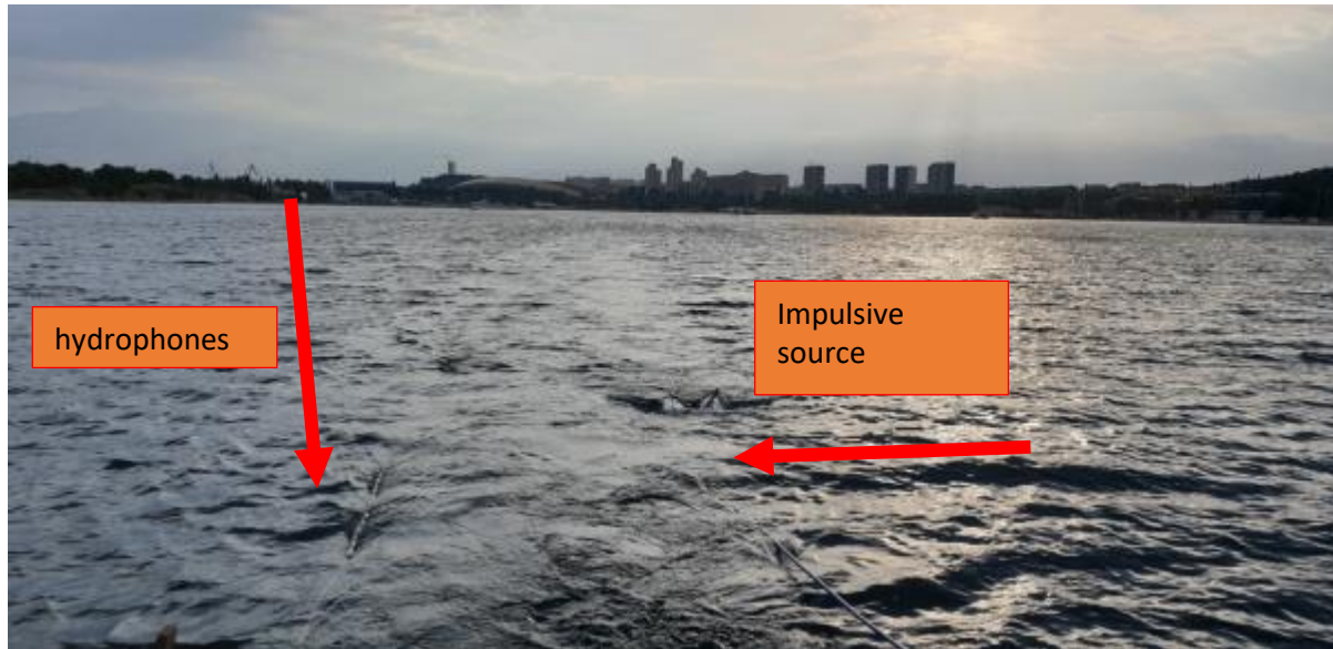
Figure 49. Boomer acquisition setup.
