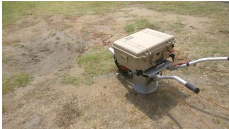
Figure 48. Top left: planted geophone. Top right: example of deployed seismic line. Bottom: vibrating source.
