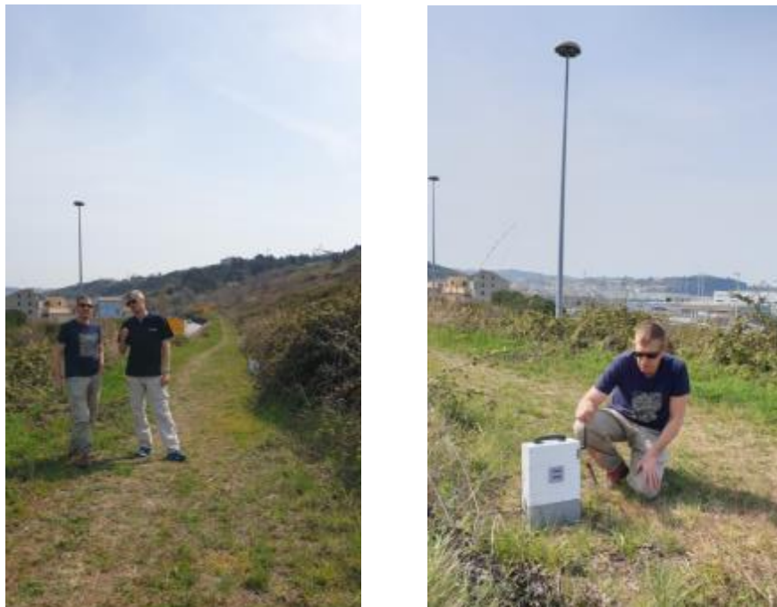
Figure 47. Left: example of geoelectrical line. Right: electrode planted in the ground and connected to a wireless transceiver.
