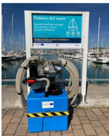
Figure 6.3.7 Mobile pump for boat black waters in marina Dorica
