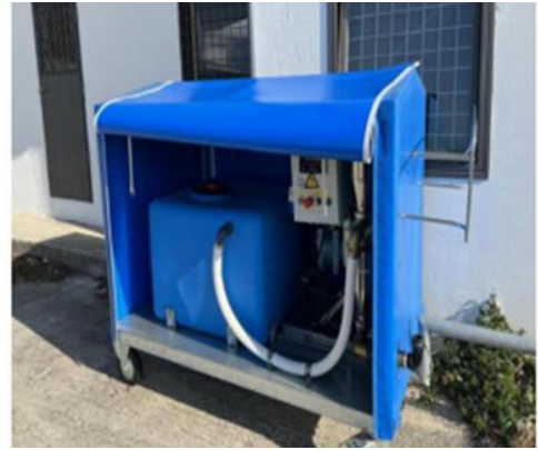
Figure 6.3.4 Mobile device for receiving and pumping fecal water from ships in marina Strožanac
