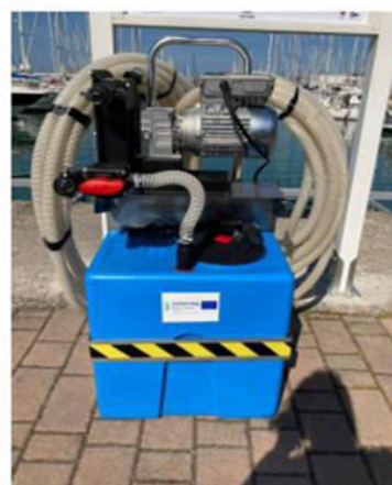
Figure 6.3.7 Mobile pump for boat black waters in marina Dorica
