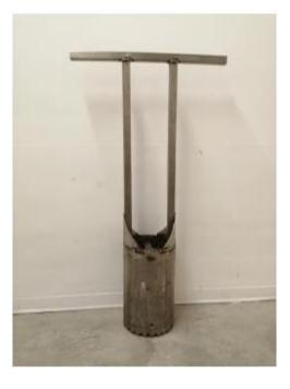
Figure 8. A typical steel core drill to extract C. nodosa sods from the donor site to transplant them in the acceptor sites.
