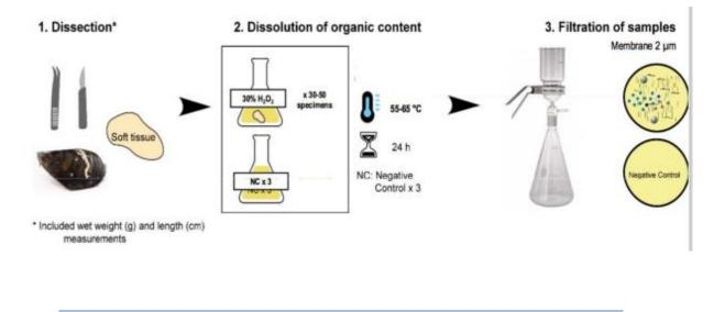
Figure 20: Laboratory procedure
