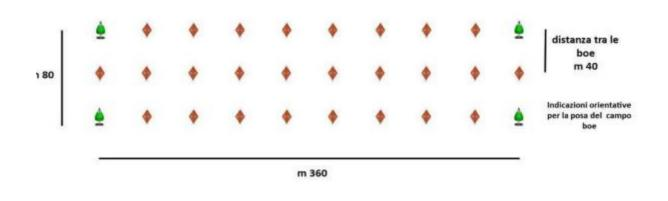
Figure 4. Buoy field and indicative representations for the functional positioning of the single mooring points.
