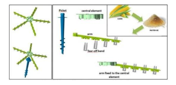
Figure 6. The biodegradable (Mater-Bi®) modular system used to anchor P. oceanica shoots to the substrate. On the left a general view of the star-shaped anchoring staple; on the right details of its components.
