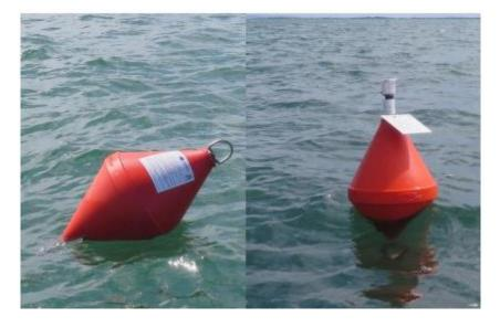
Figure 5. Buoys positioned at Monfalcone, in Panzano bay. On the left, an ordinary buoy and, on the right, a corner buoy, with lighting device.
