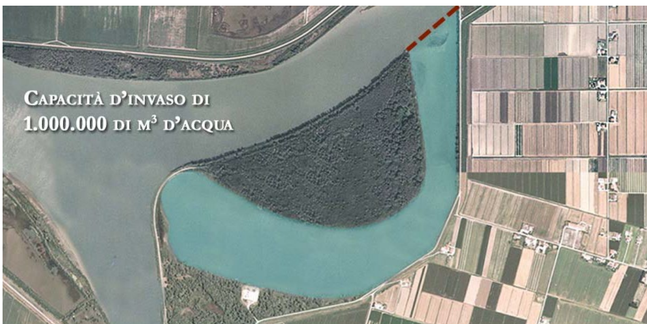
Fig. 15 – Artificial fresh water basin for irrigation realized in a meander of the Po river.
