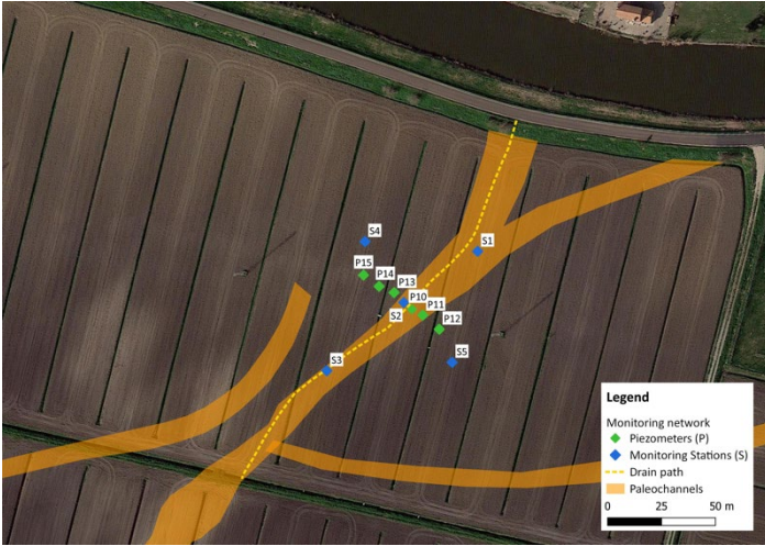
Figure 4. Map of the experimental site with the main sandy paleochannel, the drain path, and the location of the monitoring sites.
