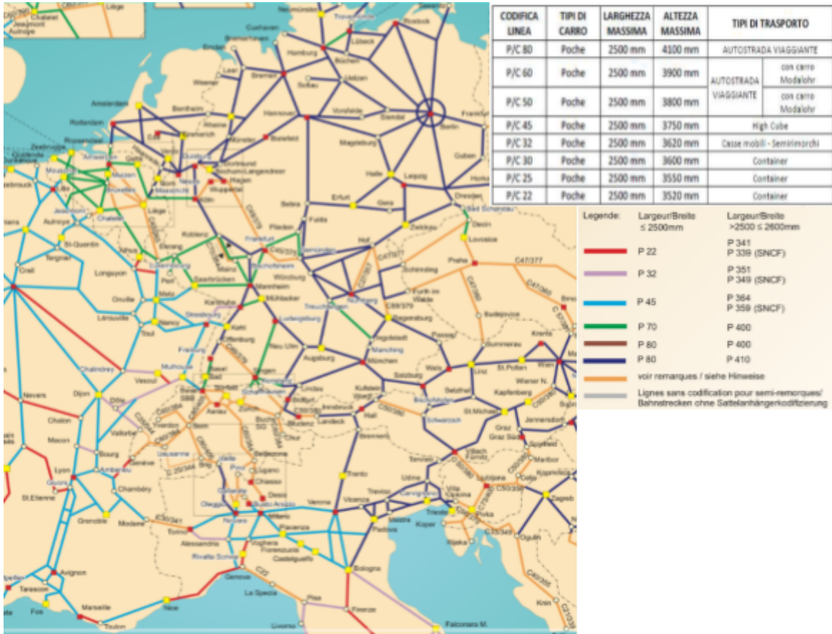
Figure 11: European railway network: loading gauge of the main lines
