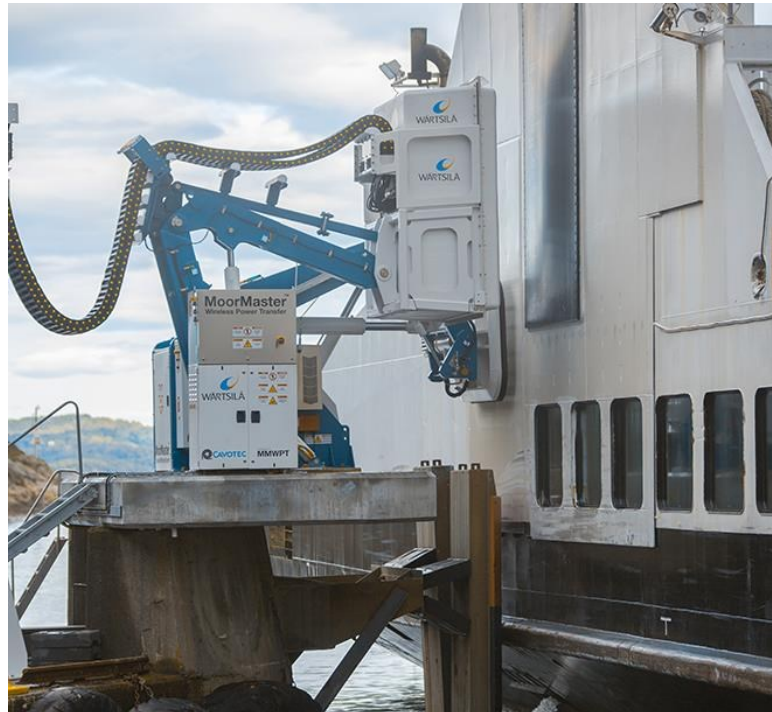
Figure 12. Example of wireless inductive connection for ferries (source: www.wartsila.com )
