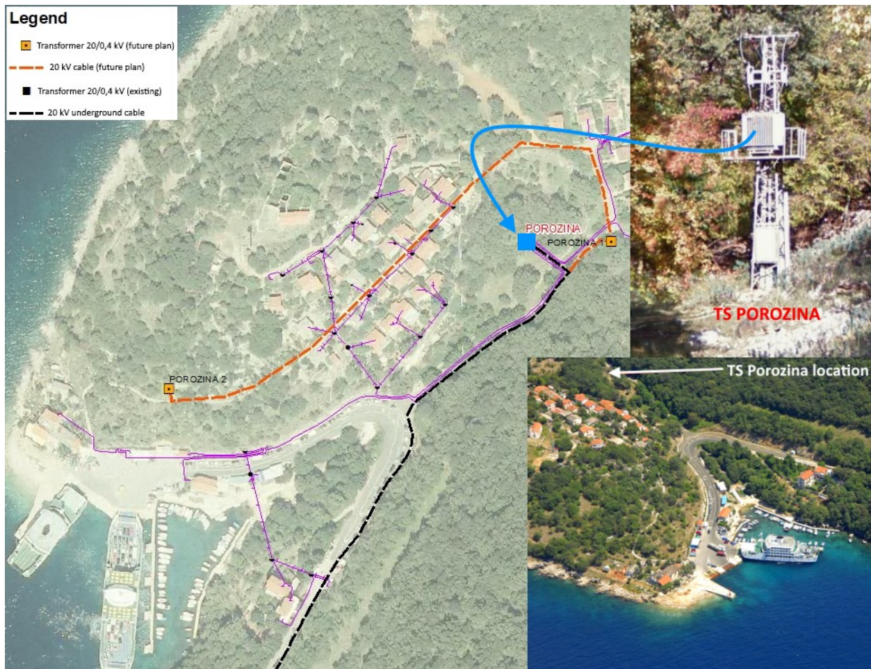
Figure9. Existing 250kVA TS and its location in Porozina
