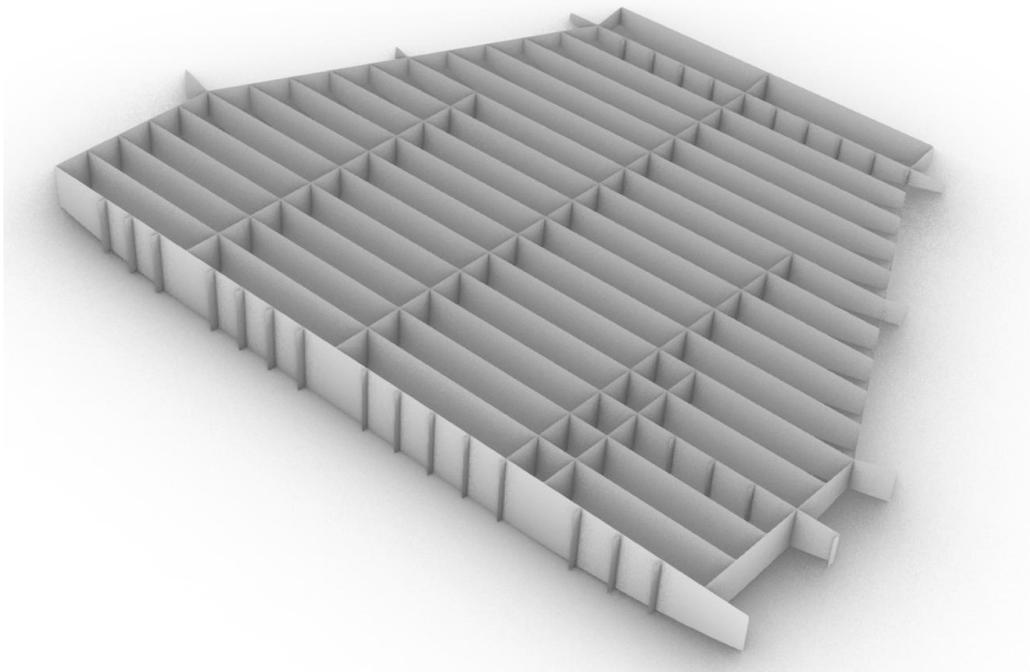
**Figure 24** *Hull geometry model – engine and battery space, bottom girders*
