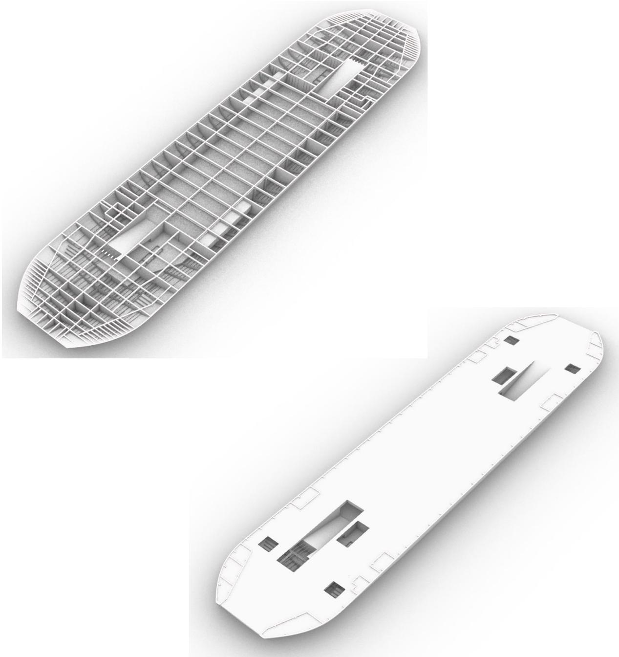
**Figure 6** *Hull geometry model - structural arrangement bellows main deck with web frames (left) and main deck (right)*
