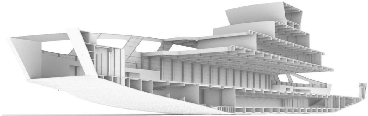
**Figure 13** *Hull geometry model – isometric view from stern-bottom*
