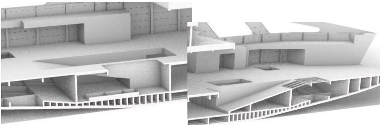
**Figure 18** Hull geometry model – for and aft driving ramps
