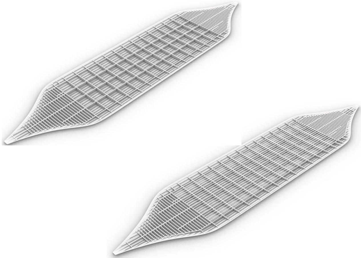
**Figure 3** Hull geometry model – double bottom bellow tank top (left)
