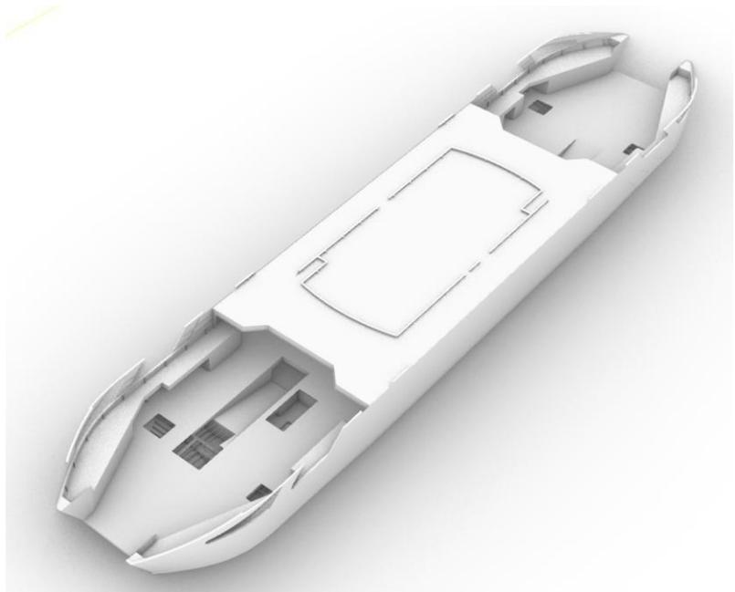
**Figure 8** Hull geometry model – structural arrangement of the passenger deck with deck transverses and longitudinals (left) and passenger deck plating (right)
