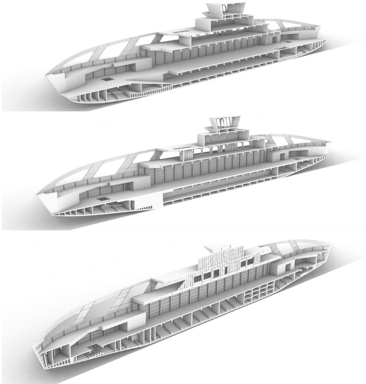
**Figure 12** *Hull geometry model – longitudinal section in CL (top) 2400 from CL (middle) and 5900 from CL (bottom)*
