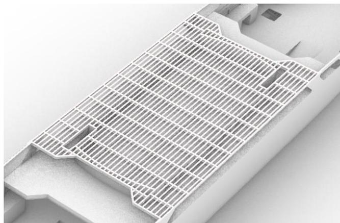
**Figure 21** *Hull geometry model – passenger deck structure*
