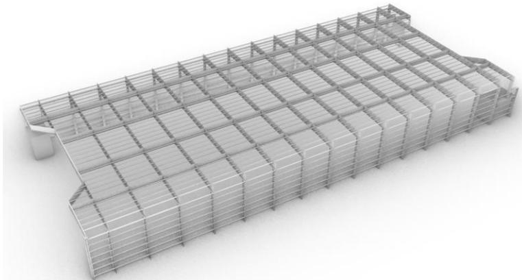
**Figure 20** *Hull geometry model – passenger deck structure*
