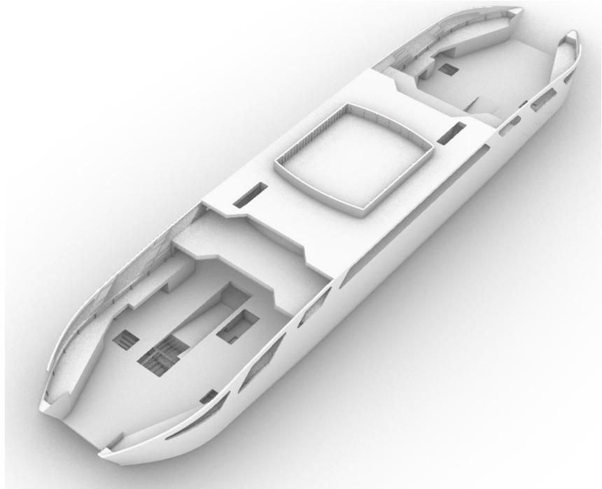
**Figure 9** *Hull geometry model – structural arrangement of the sun deck with deck transverses and longitudinals (left) and sun deck plating (right)*
