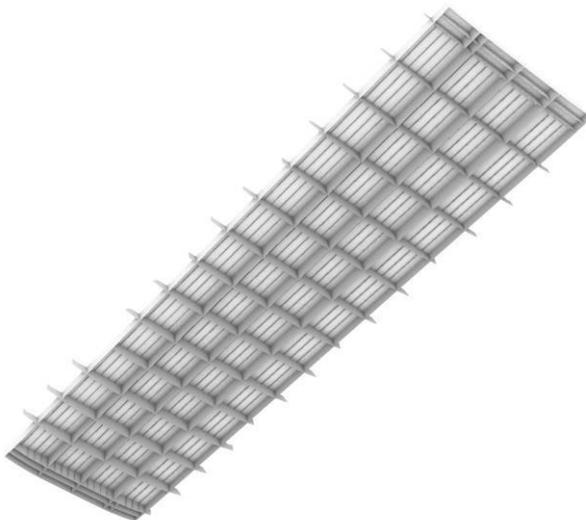
**Figure 16** *Hull geometry model – tank top structure, view from below*
