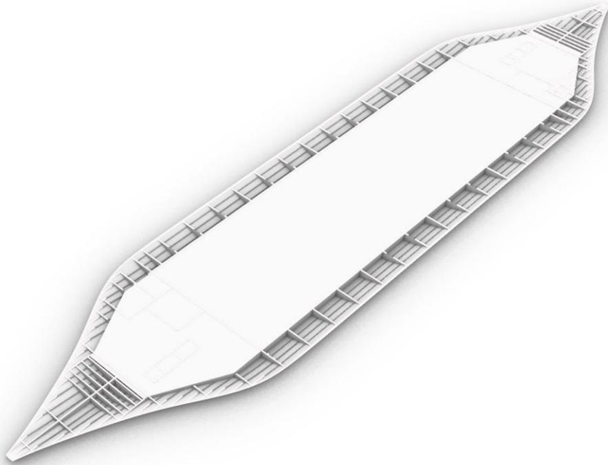
**Figure 4** *Hull geometry model – tank top*
