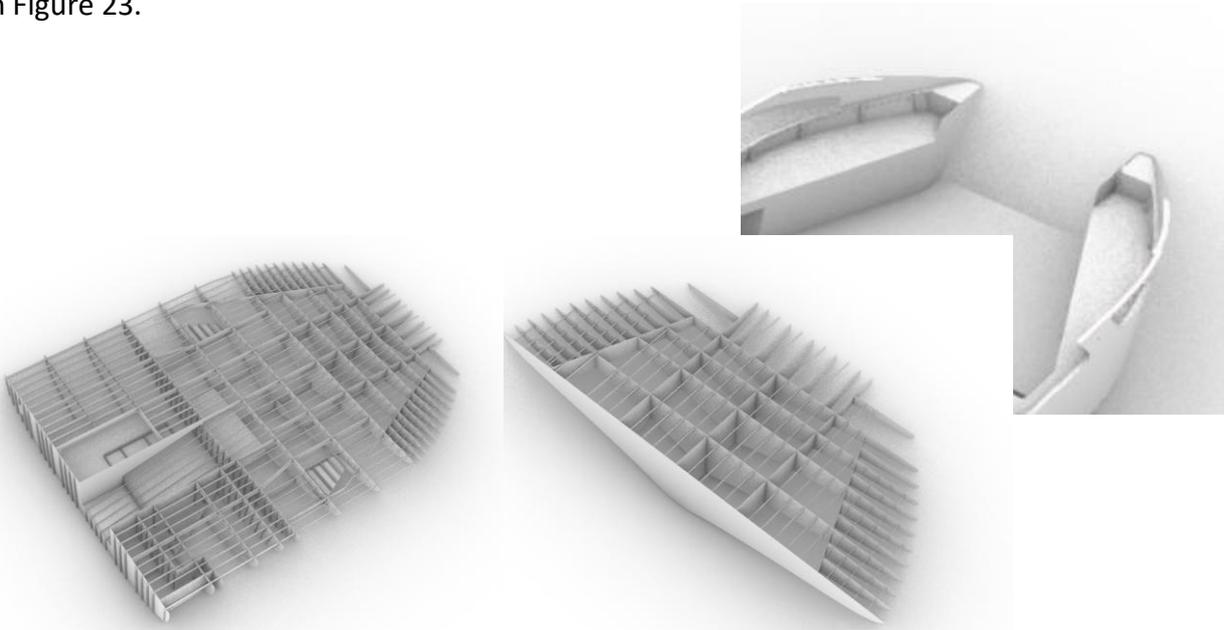
**Figure 23** *Hull geometry model – ends structure, bow stern ramps*
