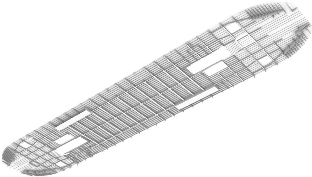
**Figure 17** Hull geometry model – main deck structure, view from below
