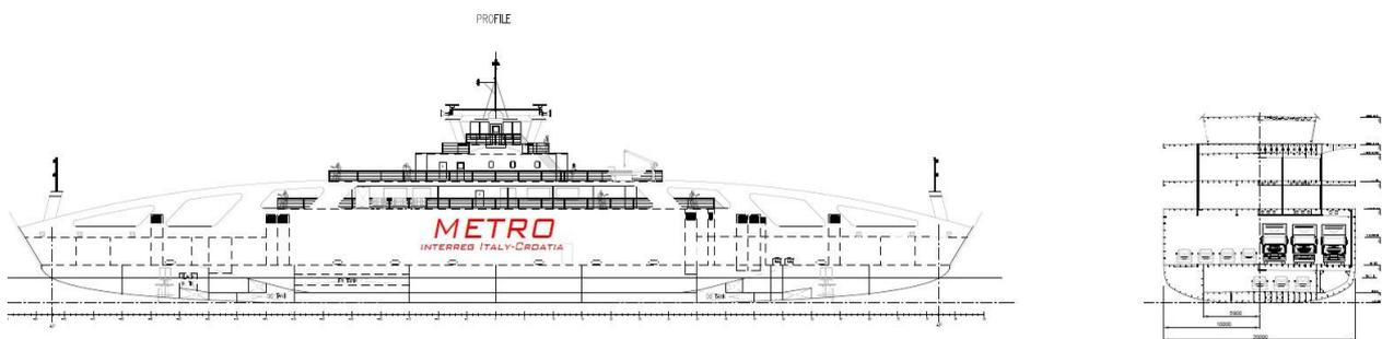
**Figure 1** General arrangement plan of double ended ferry
