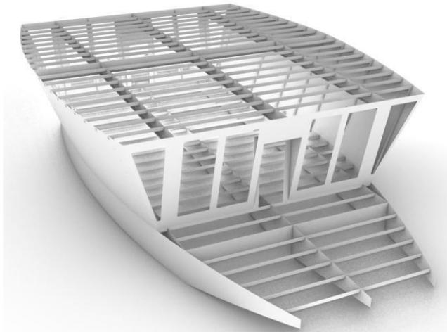
**Figure 22** *Hull geometry model – wheelhouse deck and top structure*
