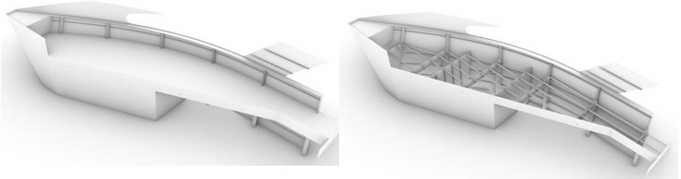
**Figure 19** *Hull geometry model – mooring and anchoring equipment deck structure (left), with plating (right)*
