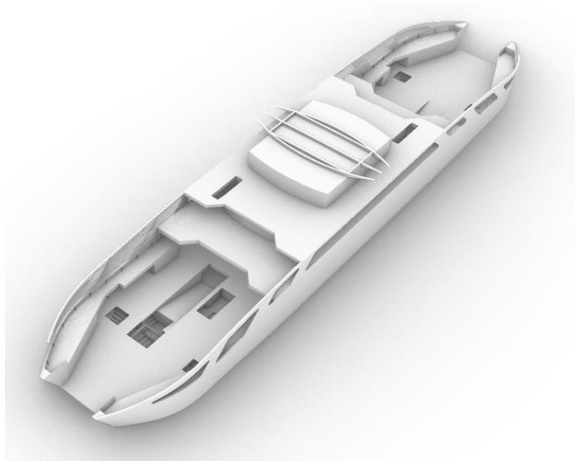
**Figure 10** Hull geometry model – superstructure top deck with deck transverses and longitudinals (left) and plating (right)
