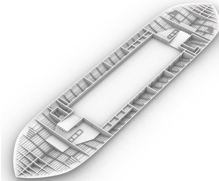
**Figure 5** *Hull geometry model – structural arrangement bellows main deck*
