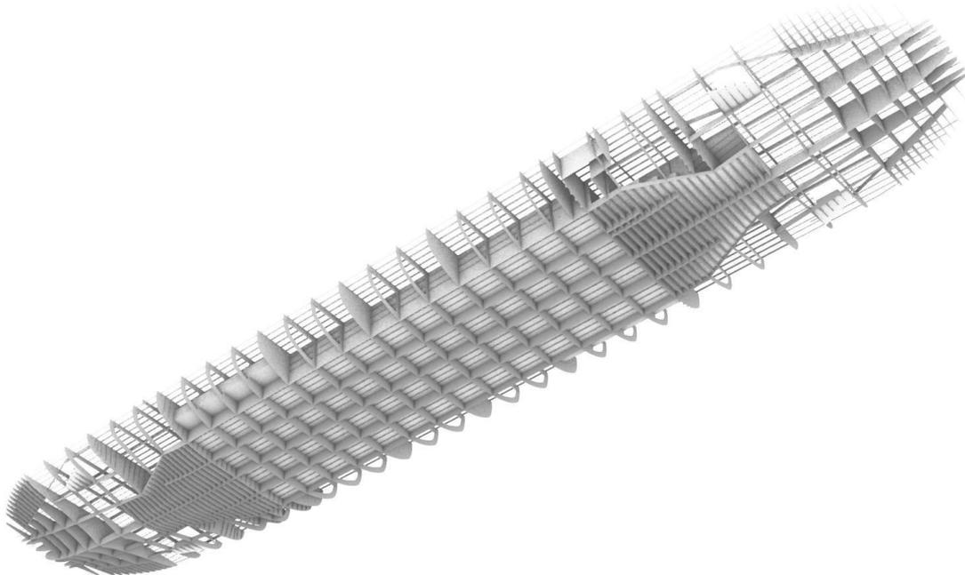
**Figure 14** *Hull geometry model – double bottom girders and longitudinals, view from below*
