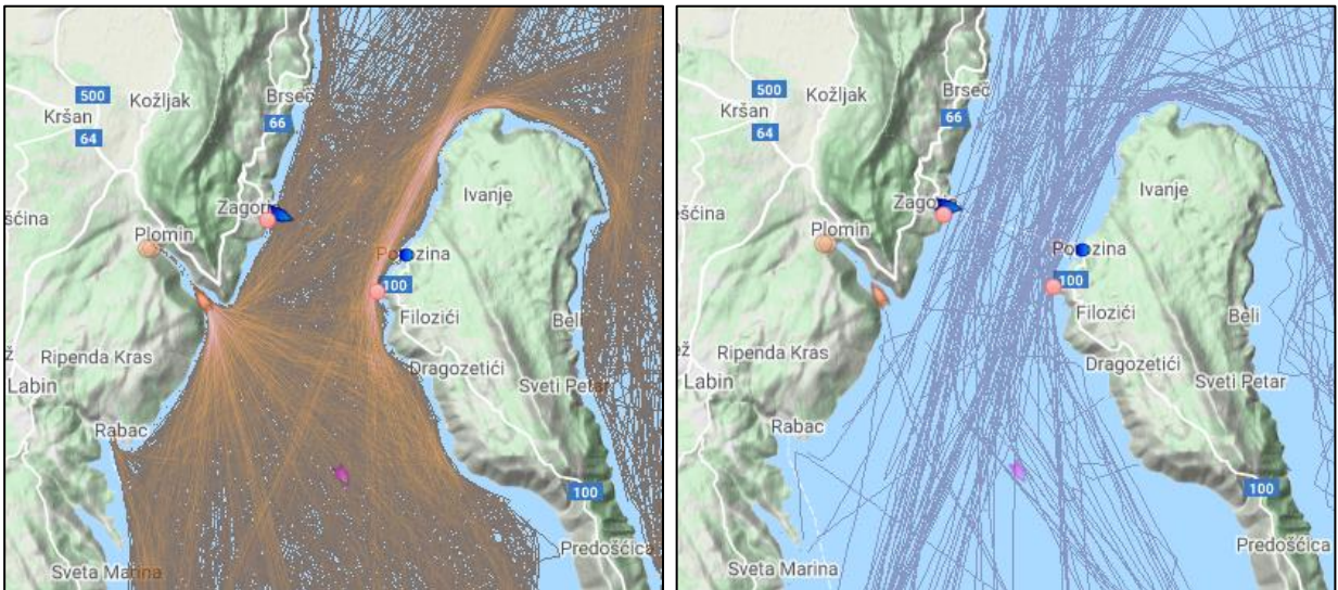
Figure 4 Fishing vessel (left) and pleasure craft (right) yearly traffic densities in Vela Vrata
