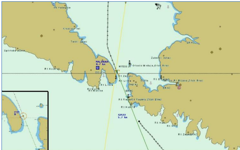
Figure 38 Record of ship Malinska (L=55,8 m) passing through Splitska Vrata (after VTS warning calls, she altered course only 150 m from shore)
