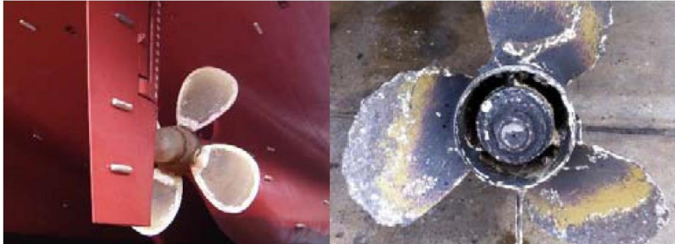
Fig. 22. In left side: Cathodic protection with sacrificial zinc anodes - In right side: corroded propeller [17].
