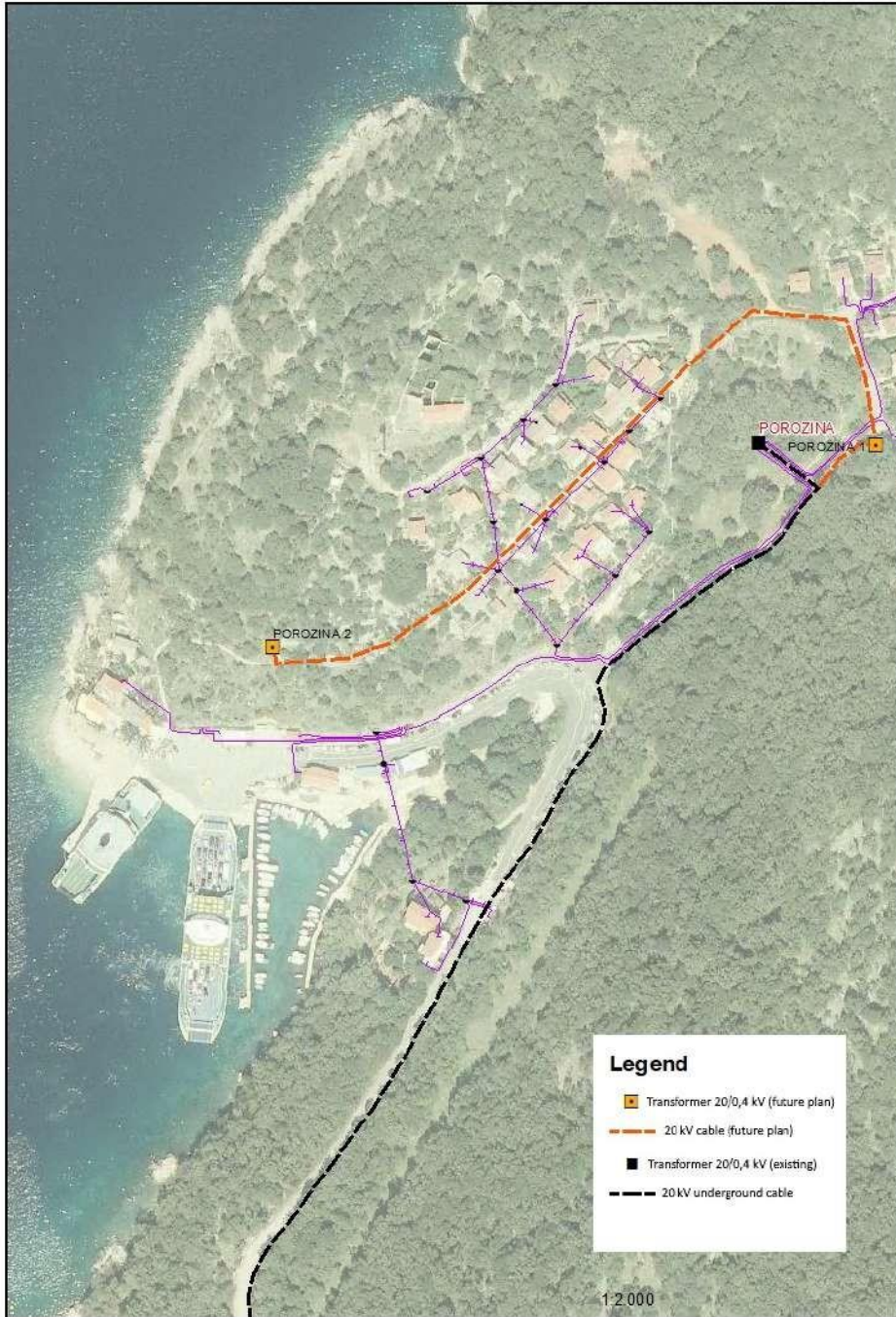
Figure 2 - Electrical power system in the Porozina port area
