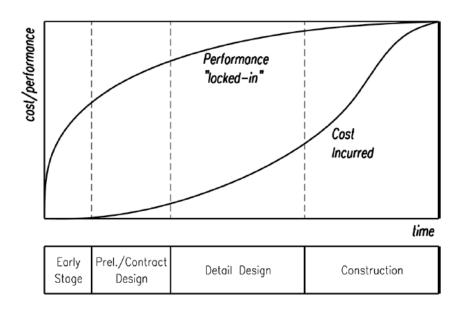
Figure 2 - Cost/performance vs time during the ship design and construction phases
