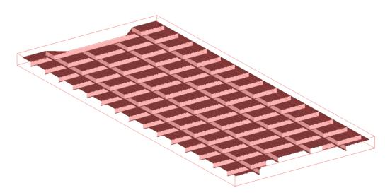
Figure 24 – Particular – 3D Passenger Deck
