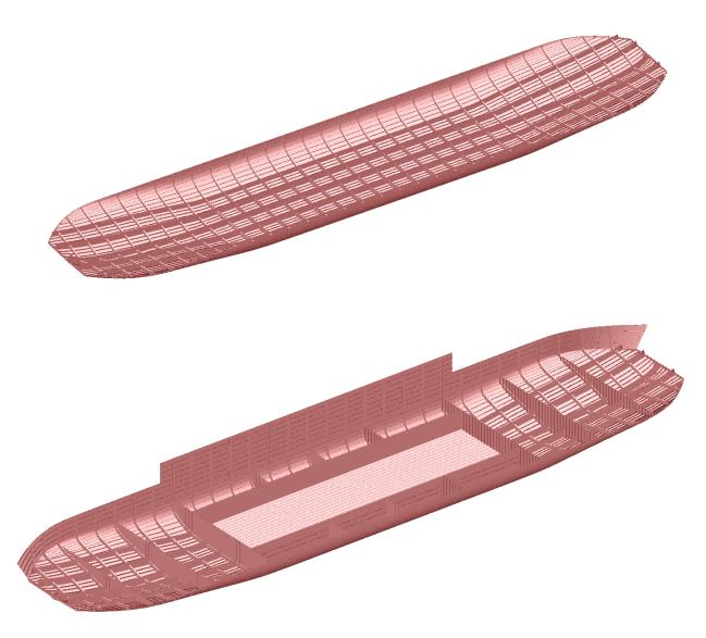
Figure 25 – Particular – Bottom's structural frame
