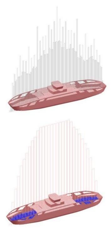
Figure 26 – Longitudinal distribution of structural (above) and vehicles (below) weight
