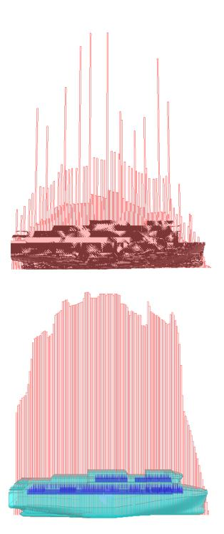
Figure 17 – Longitudinal distribution of structural (above) and cabin (below) weight
