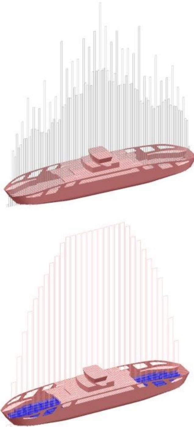
Figure 26 – Longitudinal distribution of structural (above) and vehicles (below) weight
