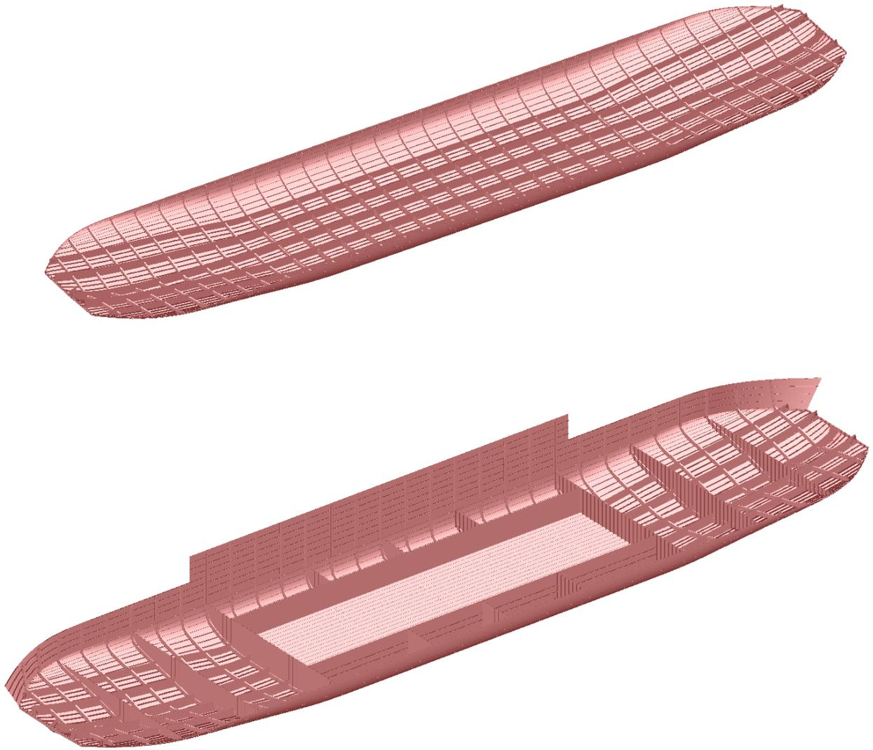
*Figure 25 – Particular – Bottom's structural frame*
