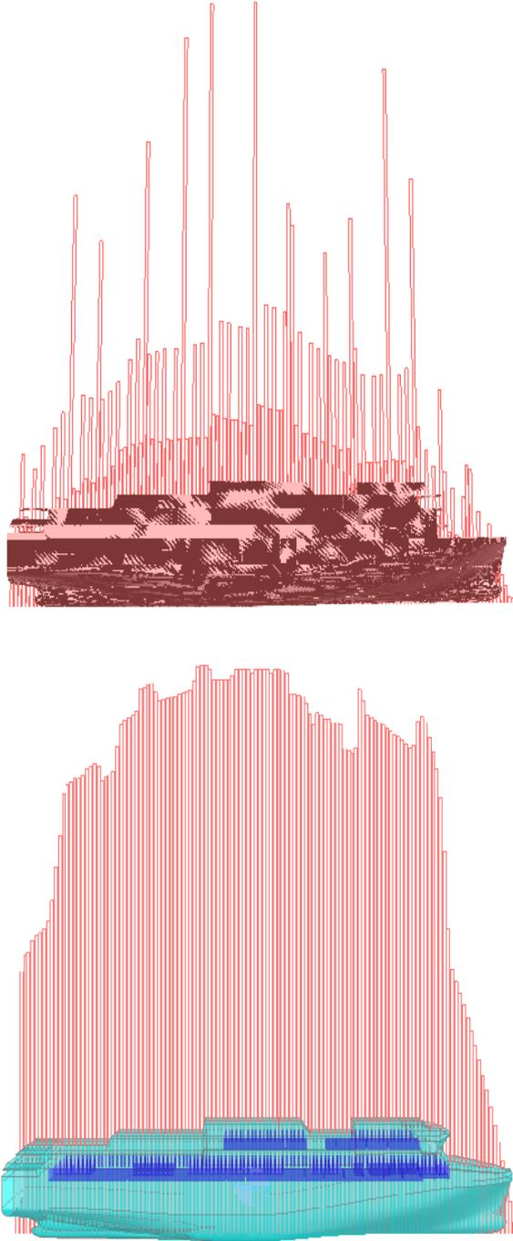
Figure 17 – Longitudinal distribution of structural (above) and cabin (below) weight
