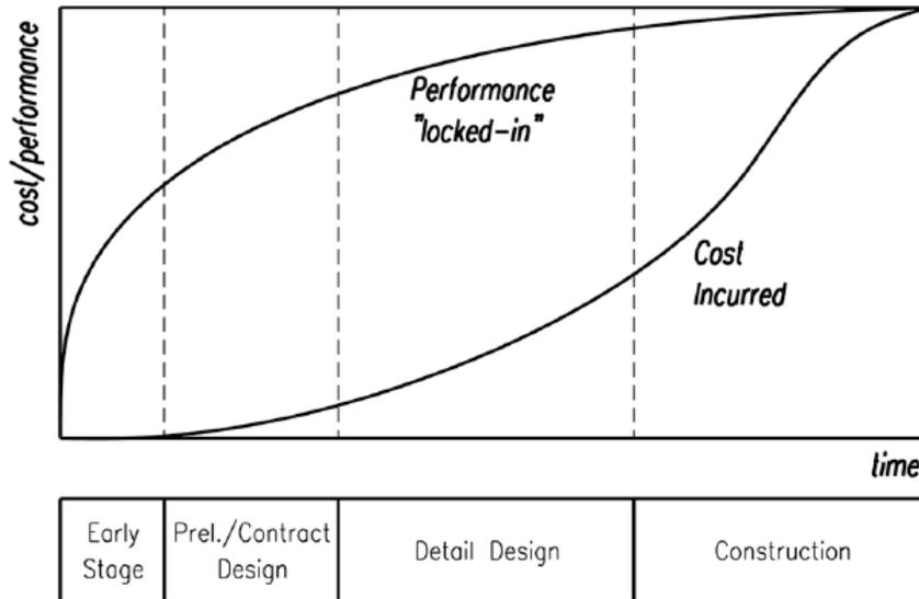
Figure 2 - Cost/performance vs time during the ship design and construction phases
