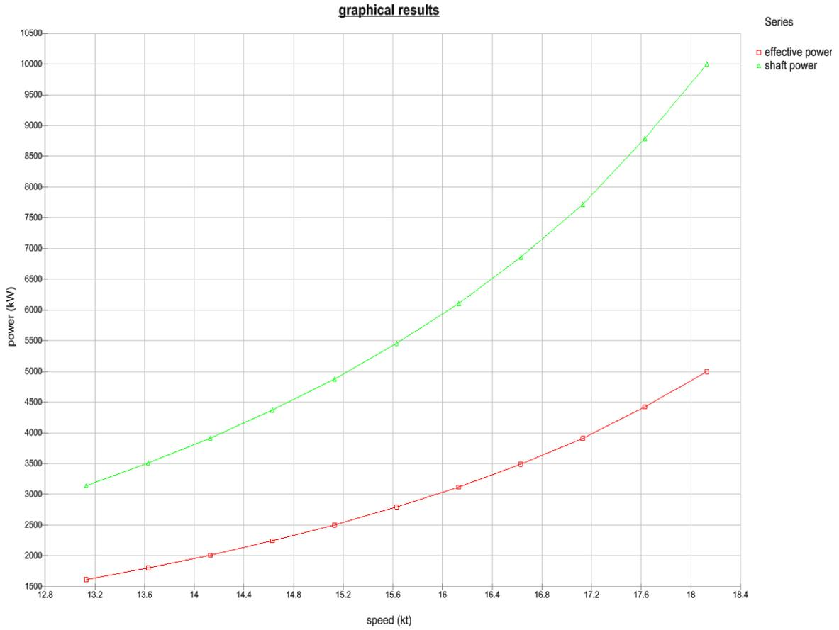
*Figure 21 – Effective and shaft power*
