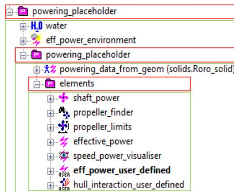
Figure 5 – Example of hierarchical system for powering: ascending (red box) and descending (green box) objects
