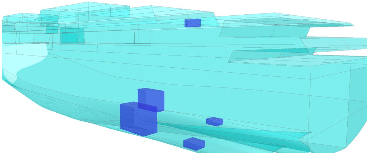
*Figure 11 – Engines and generators box models*
