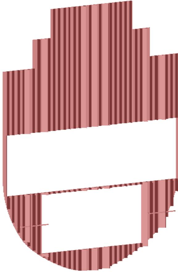
*Figure 16 – Particular – 3D Transversal bulkhead*
