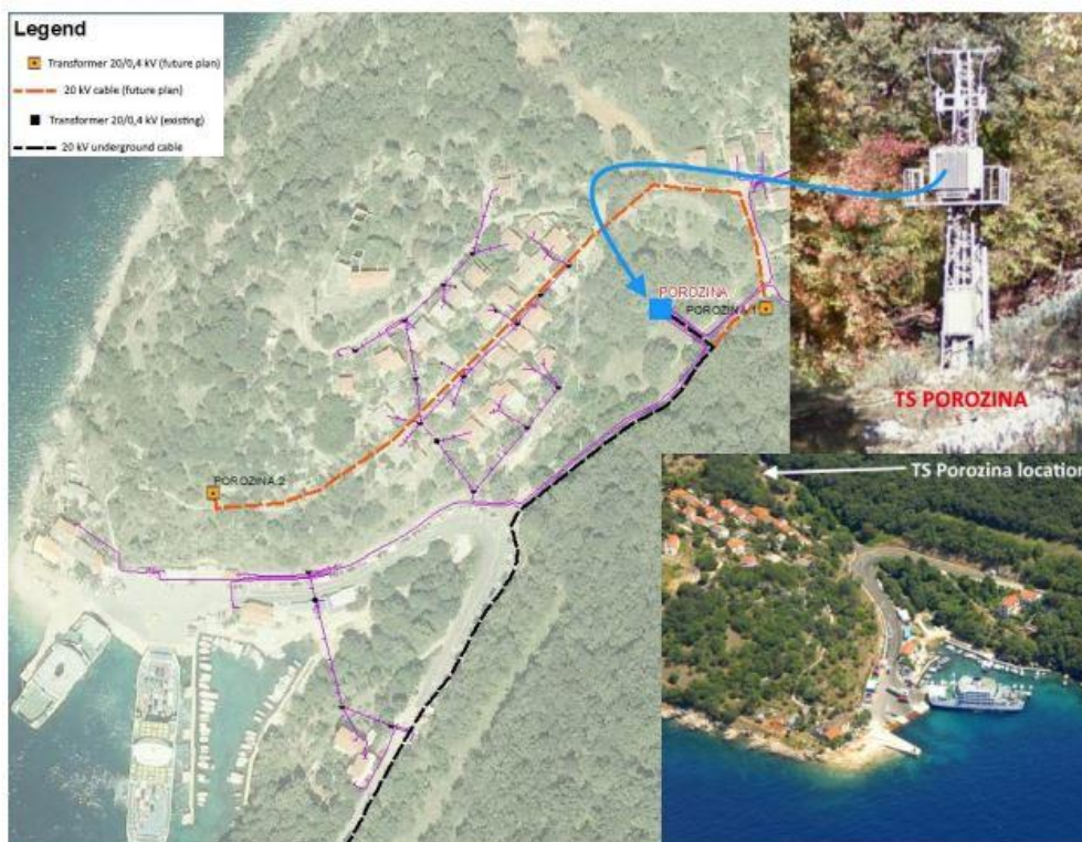
5-8 Existing 250kVA TS and its location in Porozina
