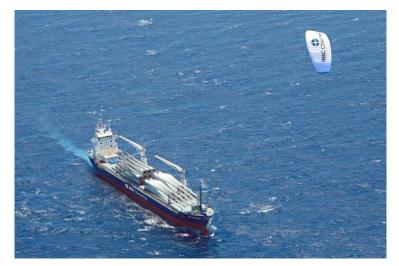
Figure 1. Towing kite system, [20]
