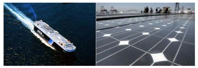
Figure 3. NYK car carrier "Auriga Leader" (left), solar panels on the top deck (right), [24]
