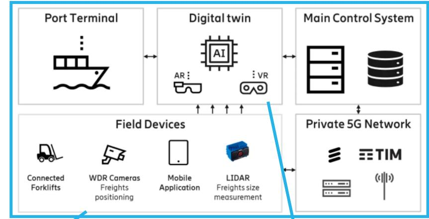
5G connected objects feed a Digital Twin engine which works in real time.
