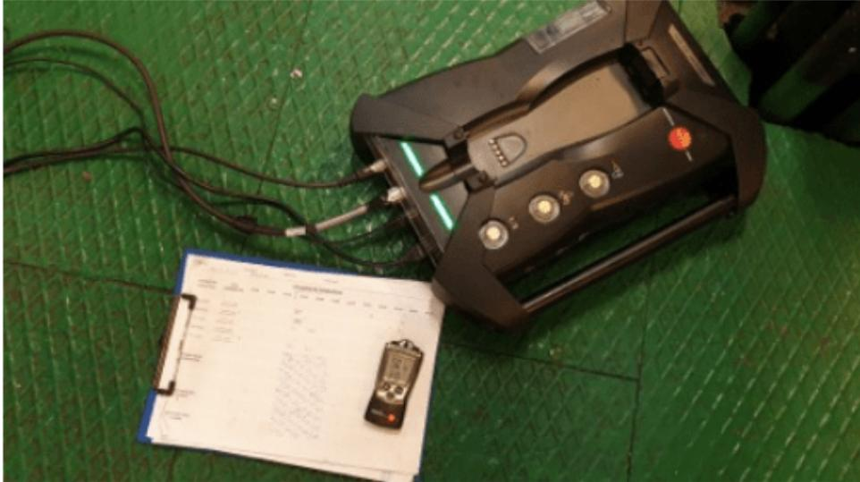
*Figure 3 TESTO 350 and the parameter data sheet*
