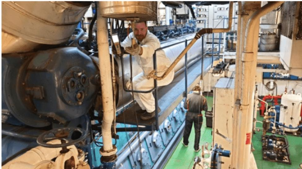
*Figure 4 Measuring the emissions and parameter recording aboard the passenger ferry ZADAR*
