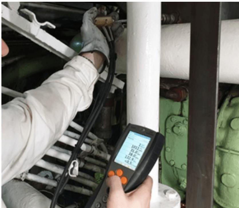
*Figure 1 Emission measurement aboard passenger ferry MARKO POLO*
