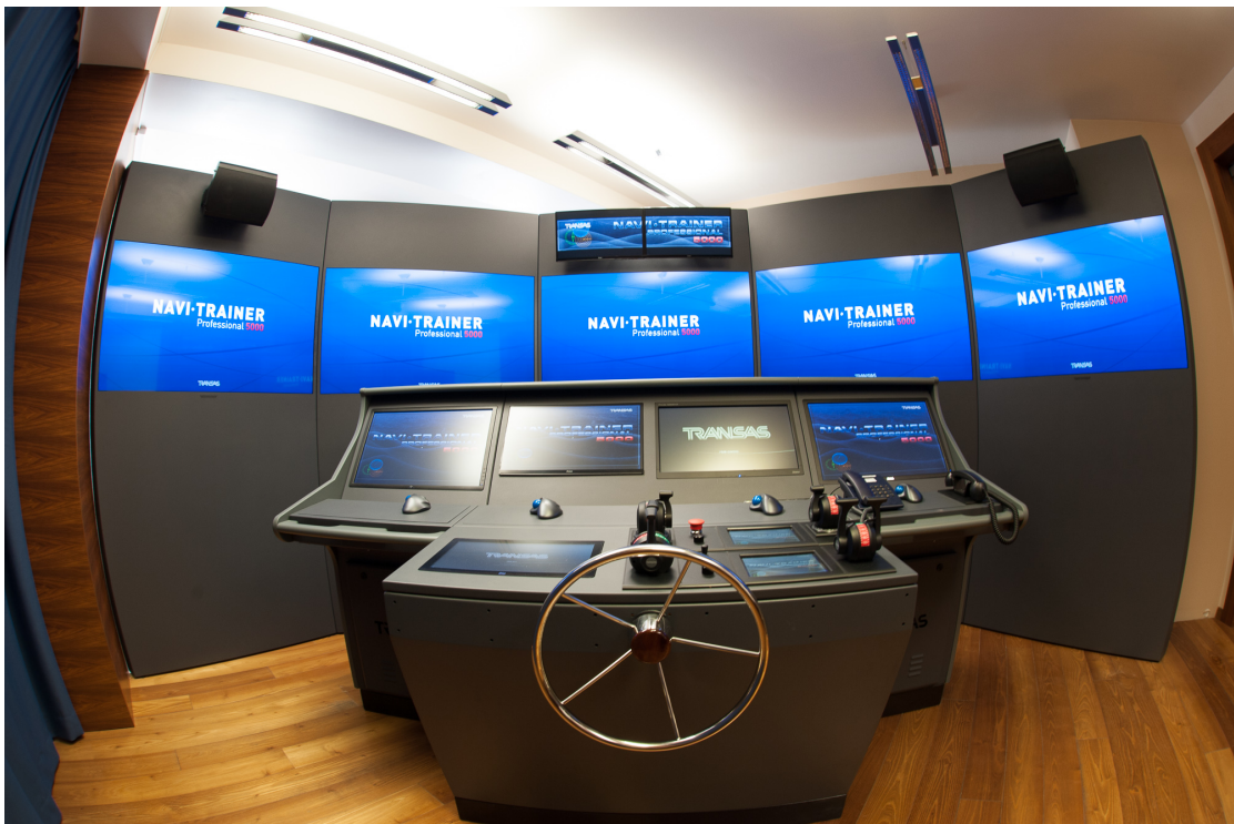
Figure 2 NTPro 5000 Navigation Simulator - command bridge console
