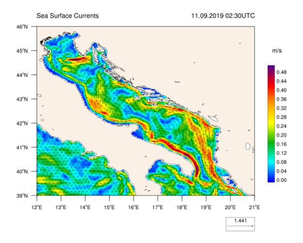
Figure 13 Example of sea surface current magnitude and direction field from MFS 1/24 degree forecast model.
