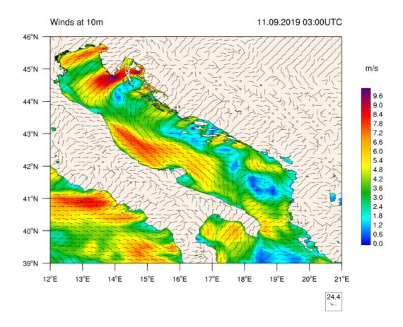
Figura 1 Example of 10m-wind magnitude and direction field from ECMWF 1/8 degree forecast model.
