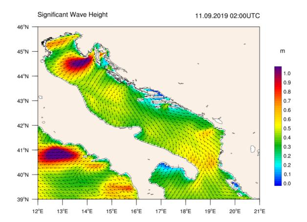
Figure 2 Example of significant wave height and direction field from WAM 1/24 degree forecast model.
