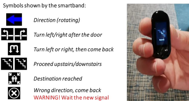
Figure 3 - Signals given by the smartband
