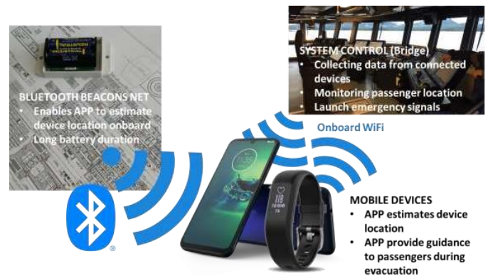
Figure 1: Schematic view of the pilot arrangement and communication between components
