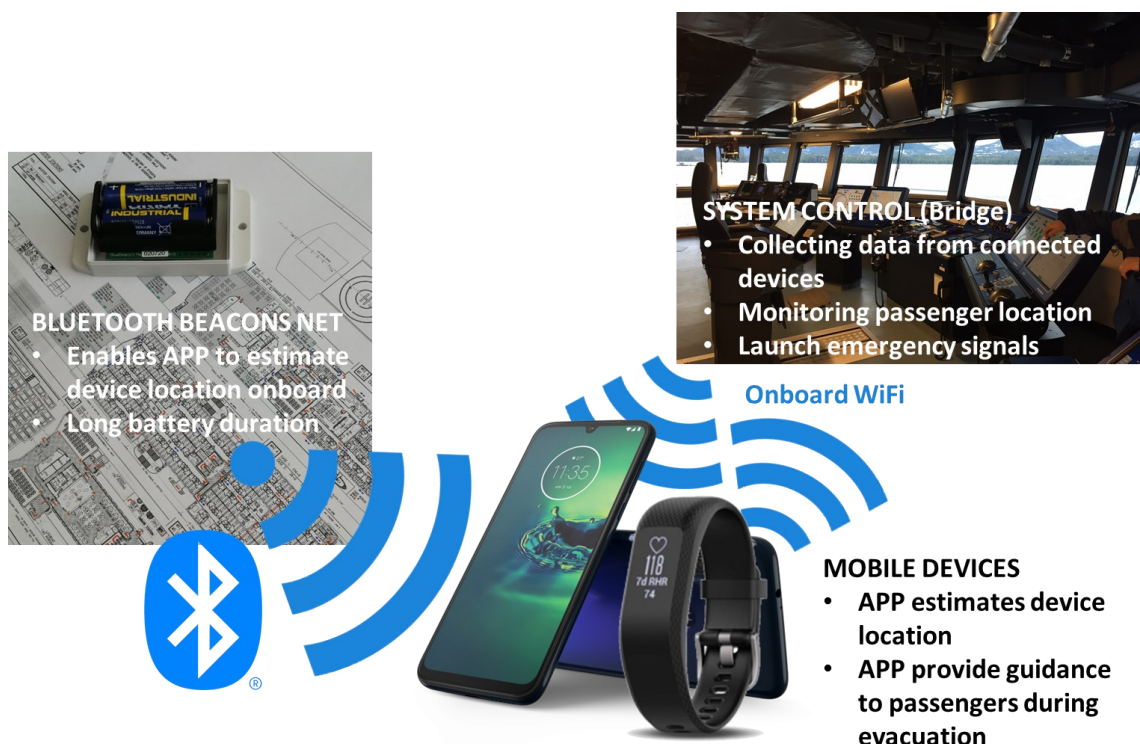
Figure 2. Schematic view of the pilot arrangement and communication between components.
