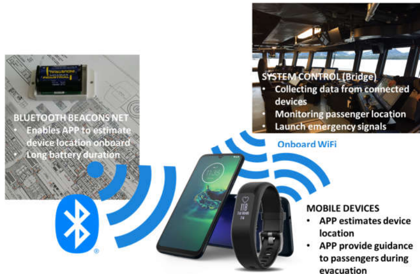
Figure 13. Schematic view of the pilot arrangement and communication between components.
