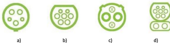
Figure 1: connectors of the different types of charging stations: a) type 1; b) type 2; c) type 4; d) CCS Combo 2
