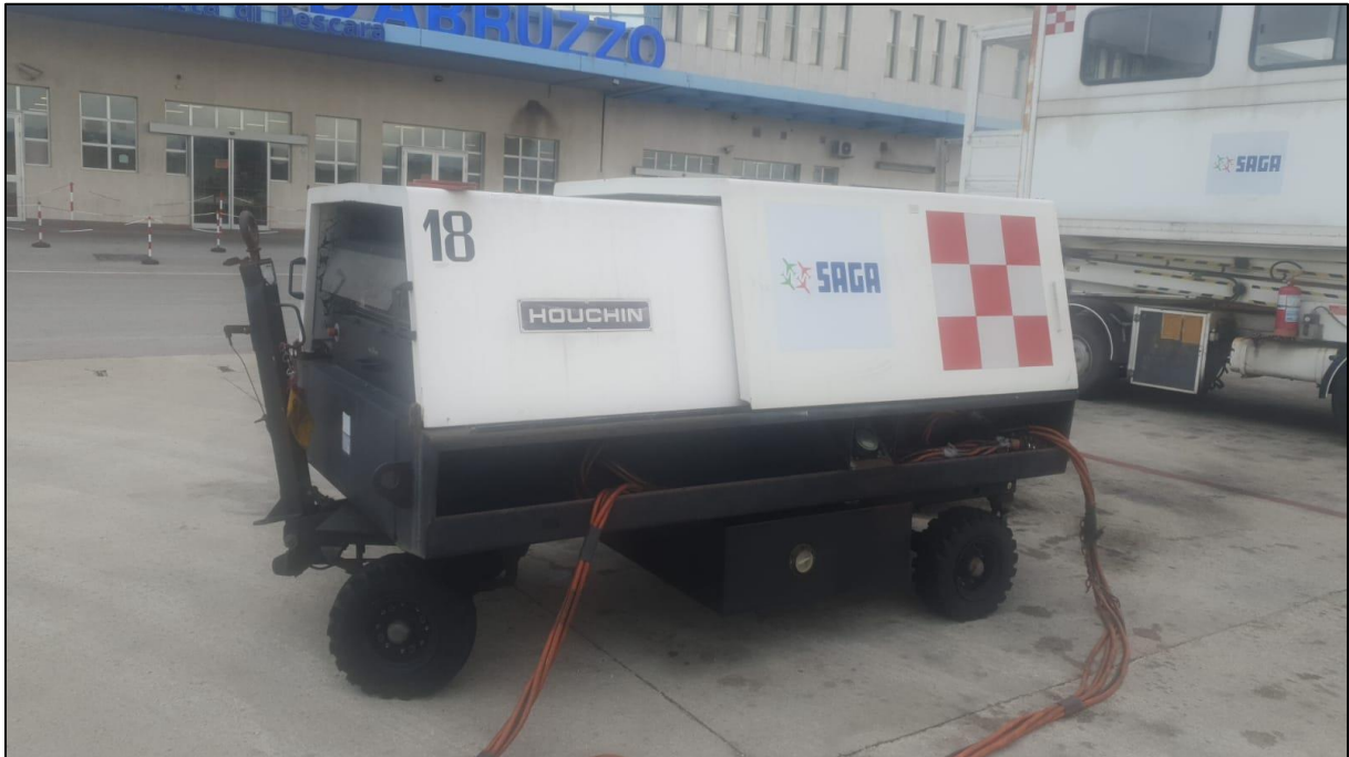
Figure 7. Diesel fuelled ground power unit replaced at Abruzzo Airport.
