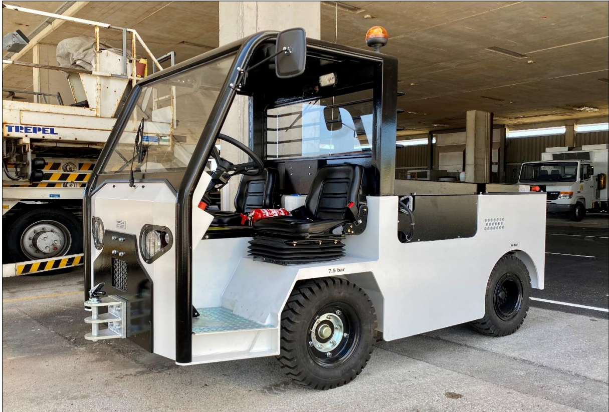
Figure 4. VET-17kN electrical towing tractor for ground handling
