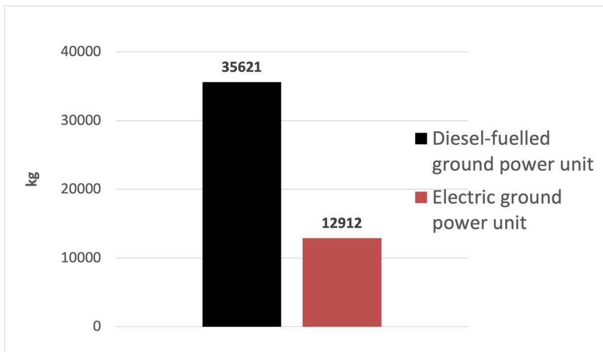
Figure 7. Comparison between greenhouse gases (CO2) emissions deriving from diesel-fuelled and electric ground power units per year.
