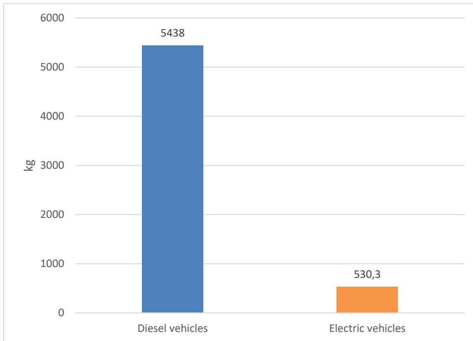
Figure 4-11. Comparison between greenhouse gases emissions deriving from diesel vehicles (CO<sub>2</sub>) and electric vehicles (CO<sub>2</sub> eq) per year, Dubrovnik port
