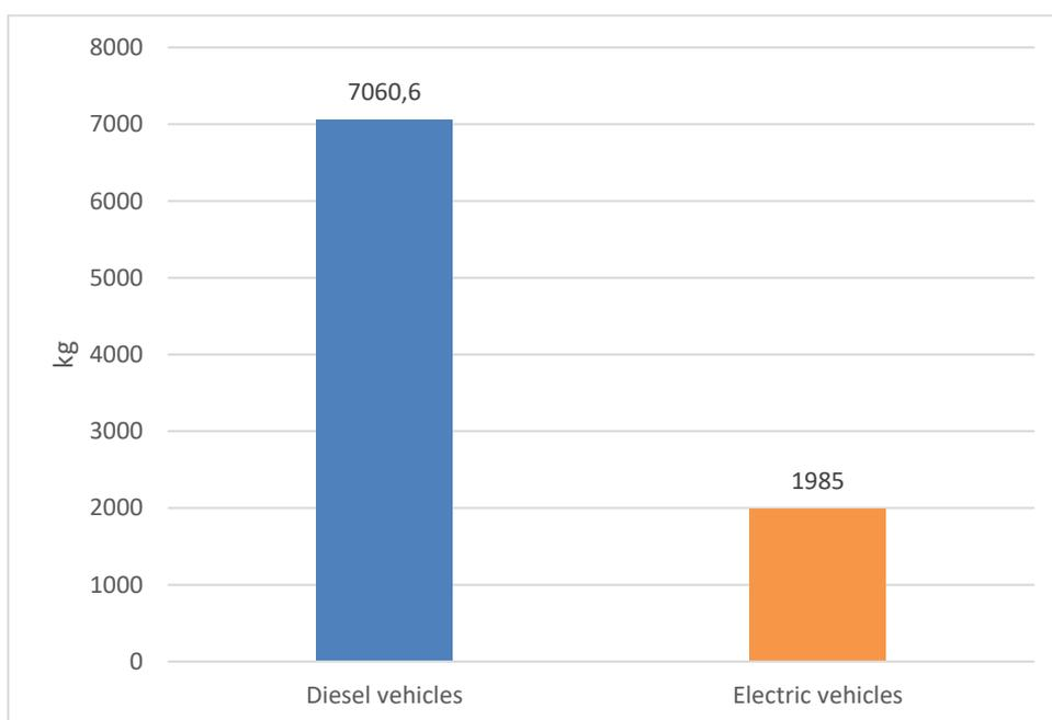
Figure 4-5. Comparison between greenhouse gases emissions deriving from diesel vehicles (CO<sub>2</sub>) and electric vehicles (CO<sub>2</sub> eq) per year, Rimini airport
