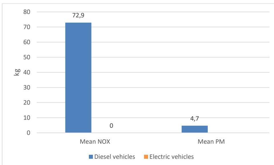
Figure 4-6. Comparison between local emissions of airborne pollutants (i.e., NO<sub>x</sub> and PM) deriving from diesel vehicles and electric vehicles per year, Rimini airport
