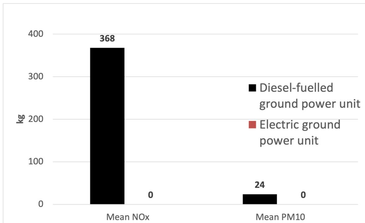
Figure 8. Comparison between local emissions of airborne pollutants (i.e., NOx and PM10) deriving from diesel-fuelled and electric ground power units per year.
