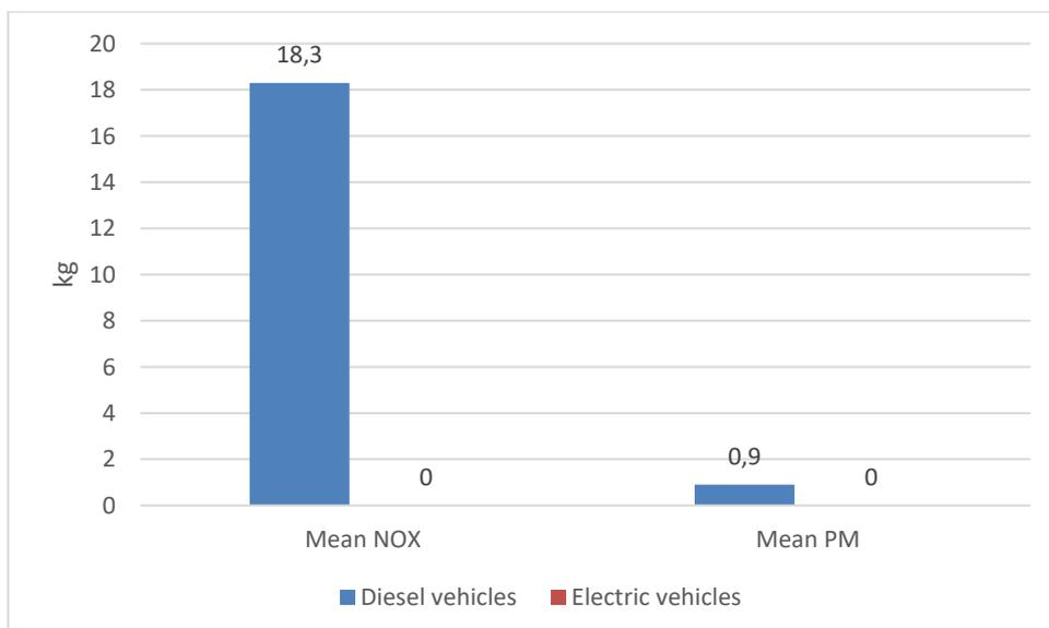
Figure 4-12. Comparison between local emissions of airborne pollutants (i.e., NO<sub>x</sub> and PM) deriving from diesel vehicles and electric vehicles per year, Dubrovnik port
