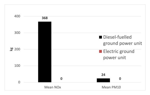
Figure 8. Comparison between local emissions of airborne pollutants (i.e., NOx and PM10) deriving from diesel-fuelled and electric ground power units per year.
