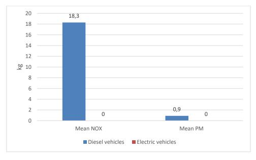
Figure 4-12. Comparison between local emissions of airborne pollutants (i.e., NOx and PM) deriving from diesel vehicles and electric vehicles per year, Dubrovnik port
