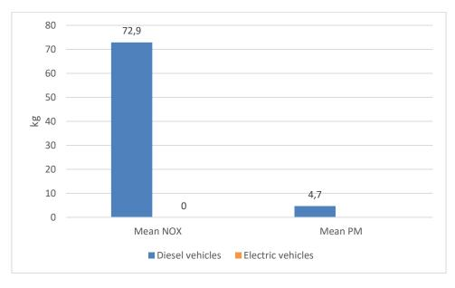
Figure 4-6. Comparison between local emissions of airborne pollutants (i.e., NOx and PM) deriving from diesel vehicles and electric vehicles per year, Rimini airport
