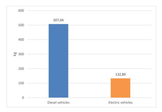
Figure 4-1. – Comparison between greenhouse gases emissions deriving from diesel vehicles (CO2) and electric vehicles (CO2 eq) per year, Brindisi airport
