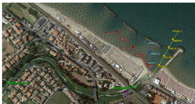
Figure 6.3 - 2 Map of seawater sampling in front of the Arzilla mouth. Sampling stations are distributed along three transects (transect 1 in red, transect 2 in blue, transect 3 in yellow) at increasing distance from the shore with different sampling points: 50m, 100m, 150m, 200m, 250m from the mouth.
