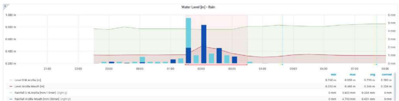
Figure 6.2 - 8 Rainfall temporal trend and river level measured in the stations of Fano Arzilla outfall and Santa Maria dell'Arzilla (about 10 km away based on ancillary data).
