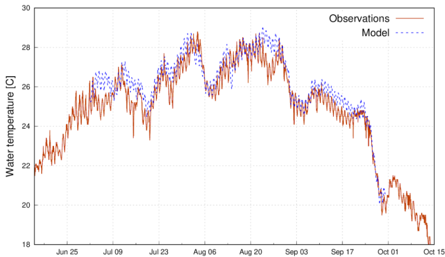
Figure 3: Measured and simulated water temperature in Pescara harbour (summer 2020).
