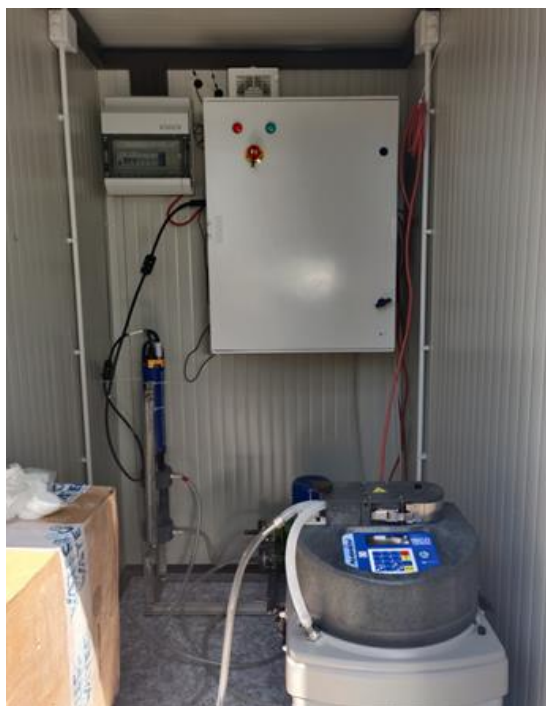
Figure 4. Real-time data acquisition system implemented at Arzilla River upstream (FANO Pilot site).
