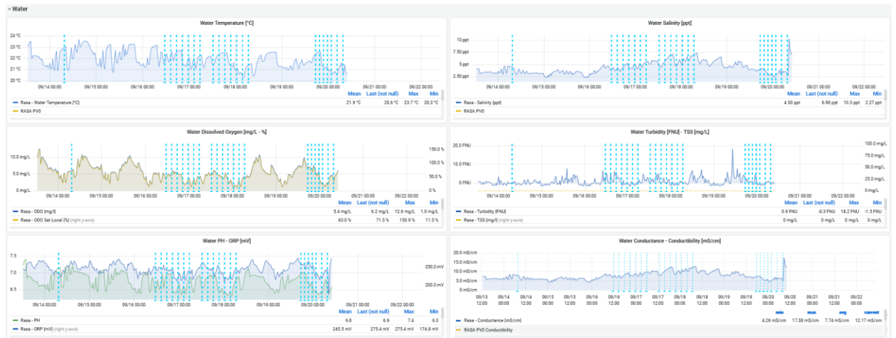
Figure 3.8.6. Example of the water section. The vertical blue lines indicate the time of river automatic sampling. They are shown in all graphs of the site dashboard.
