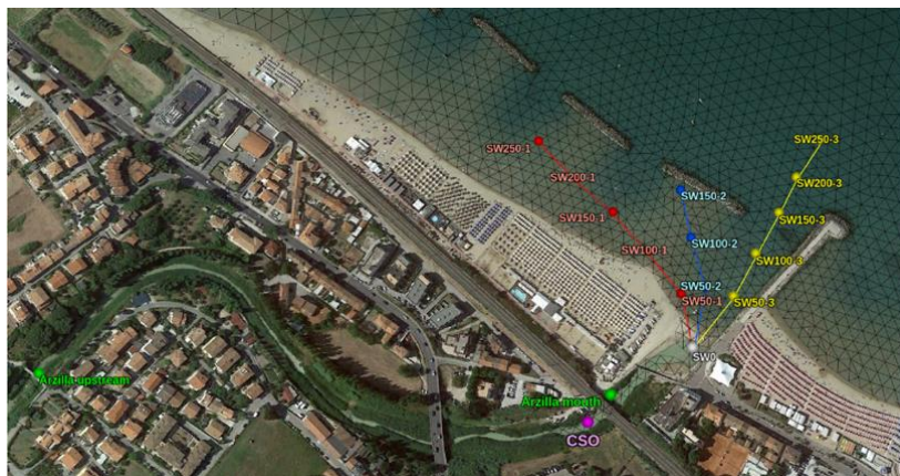
Figure 2. Map of seawater sampling in front of the Arzilla mouth. Sampling stations are distributed along three transects (transect 1 in red, transect 2 in blue, transect 3 in yellow) at increasing distance from the shore with different sampling points: 50m, 100m, 150m, 200m, 250m from the mouth.
