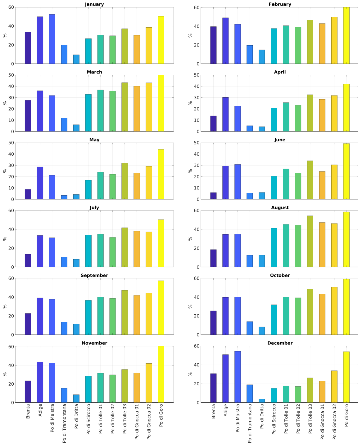
Figure 18: PS1 – Po Delta. Monthly percent of released particles that can potentially beach computed over the whole simulated period (2015–2018) for the whole pilot site (red bar) and for each river mouth
