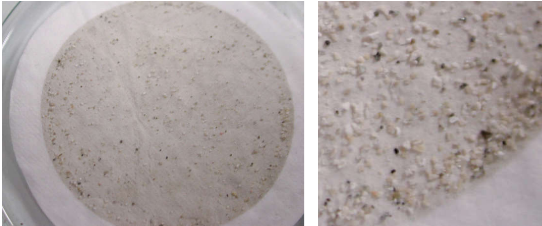
Figure 5 – sample picture of a filter and details of filter surface: several “grains” are noticeable
