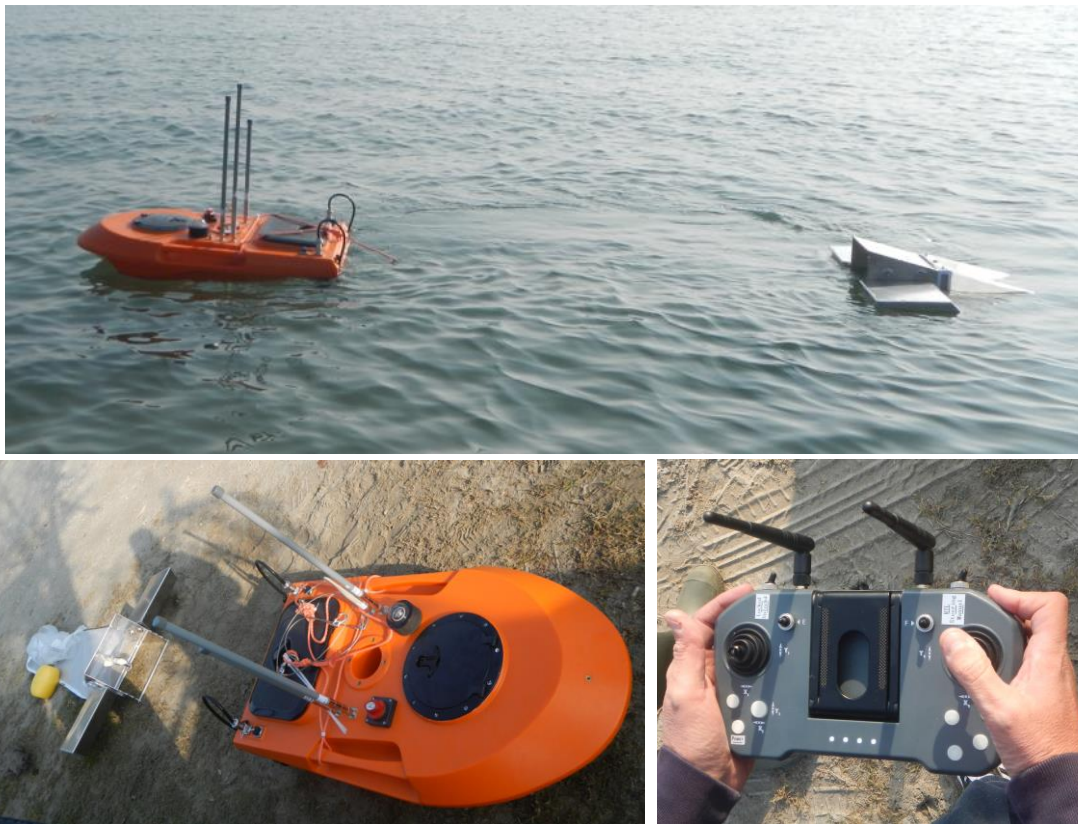
Drone and mini-manta at sea and on land. Drone remote console
