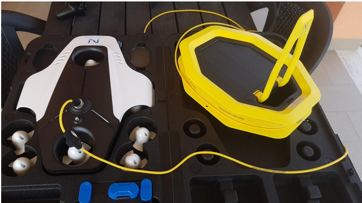
Drone – Buoy Tether Connection
