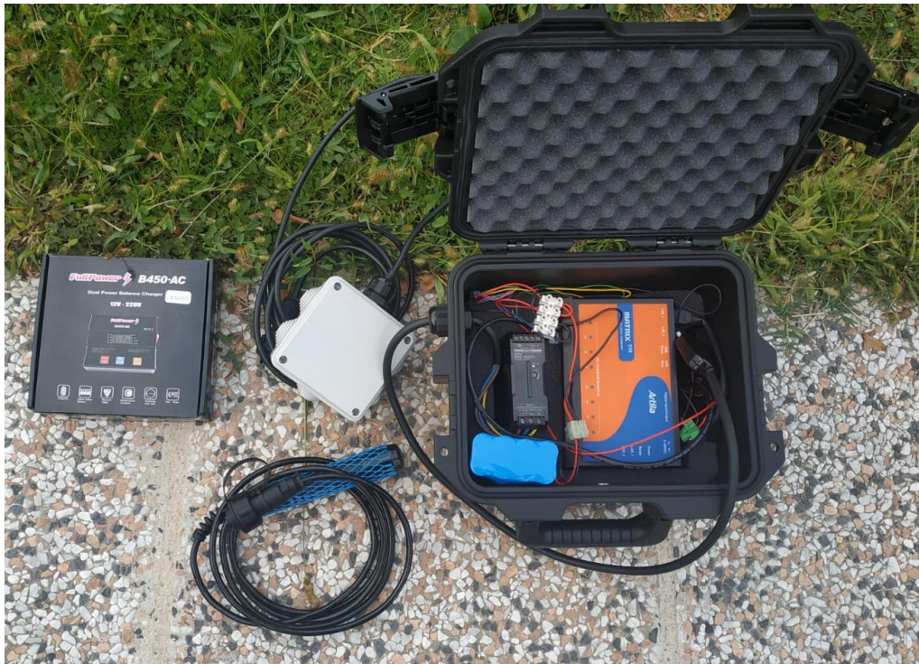
OBU: datalogger box, CT and GNSS, battery charger
