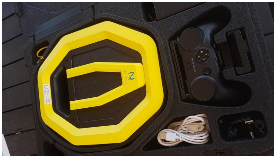
Wireless Surface Relay Buoy – Controller – Buoy Charging Cables
