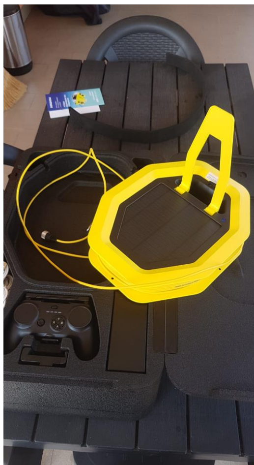
Wireless Surface Relay Buoy Switched On (Antenna up)
