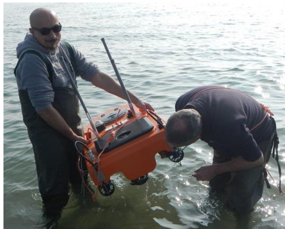
HOLO2 sensor mechanically fixed under the drone hull
