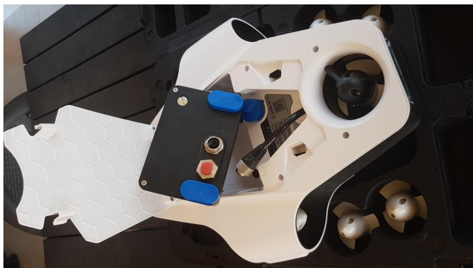
Flipped up drone with opened battery housing
