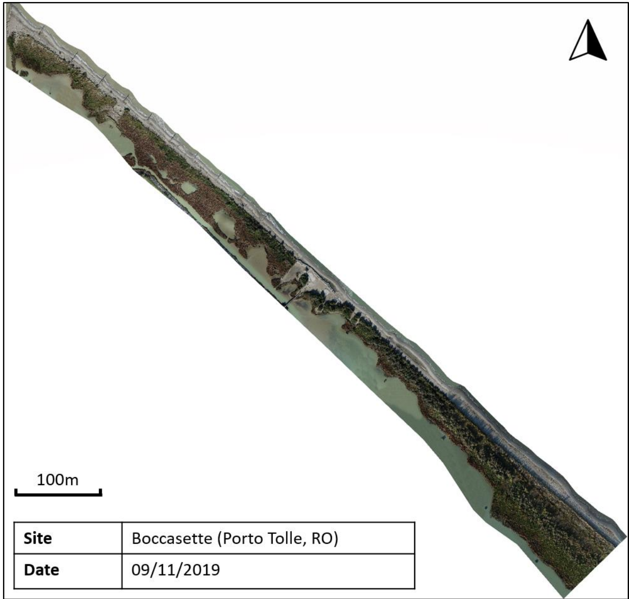
Figure 47: Example of drone imaging elaboration: orthophoto of Boccasette (flying height 50m).
