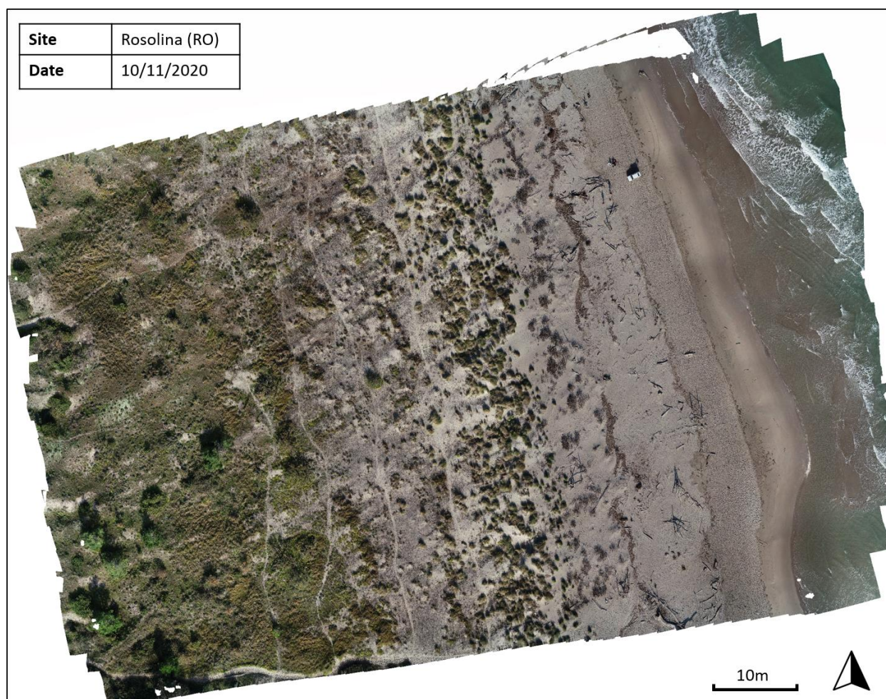
Figure 49: Example of drone imaging elaboration: orthophoto of Rosolina (flying height 25m).
