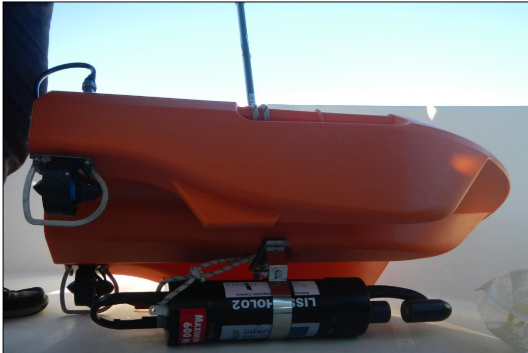
Figure 27: LISST-HOLO Sequoia sensor, mounted below the marine drone.
