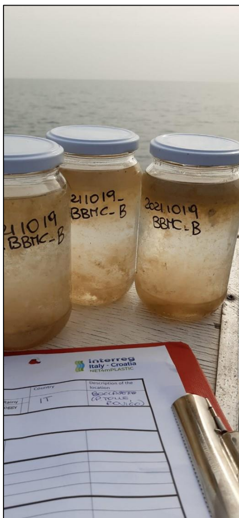
Figure 23: Sample collected and stored in 3x500 ml glass jars properly labelled (already added with ethanol 70%).
