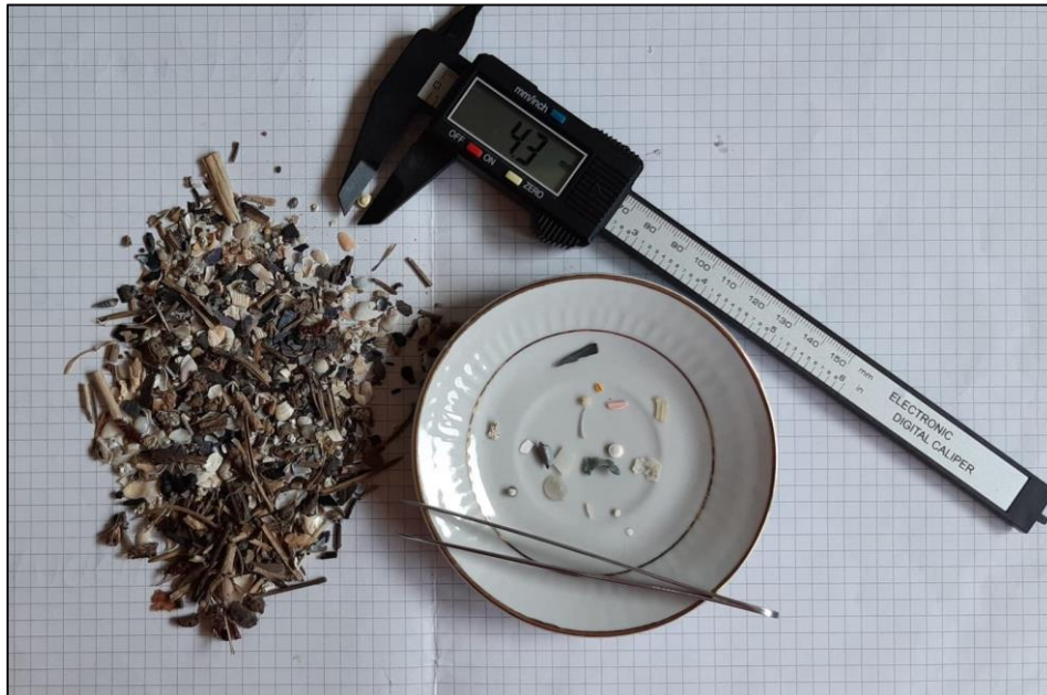
Figure 15: Manual sorting of LMP items from other particles and measure of LMP items with electronic digital calibre.
