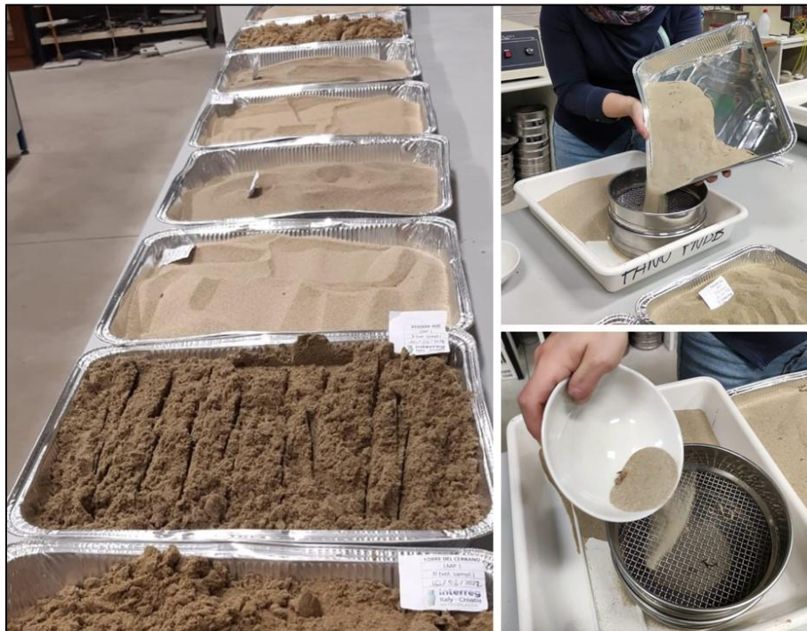
Figure 14: Example of LMP's wet sample air-dried and sieved in laboratory.
