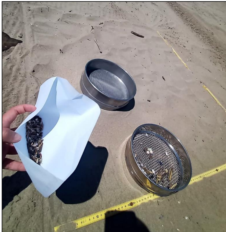
Figure 13: Example of LMP's dry sample sieved in situ (through 5 mm and 1 mm mesh size sieves) and stored in paper bags.
