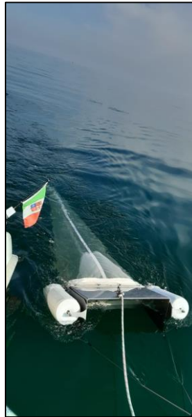
Figure 19: The manta net deployed at the side of the vessel, out of the wake zone.
