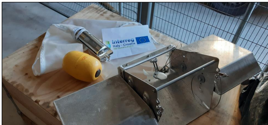
Figure 28: “Mini-manta” dragged by the marine drone.
