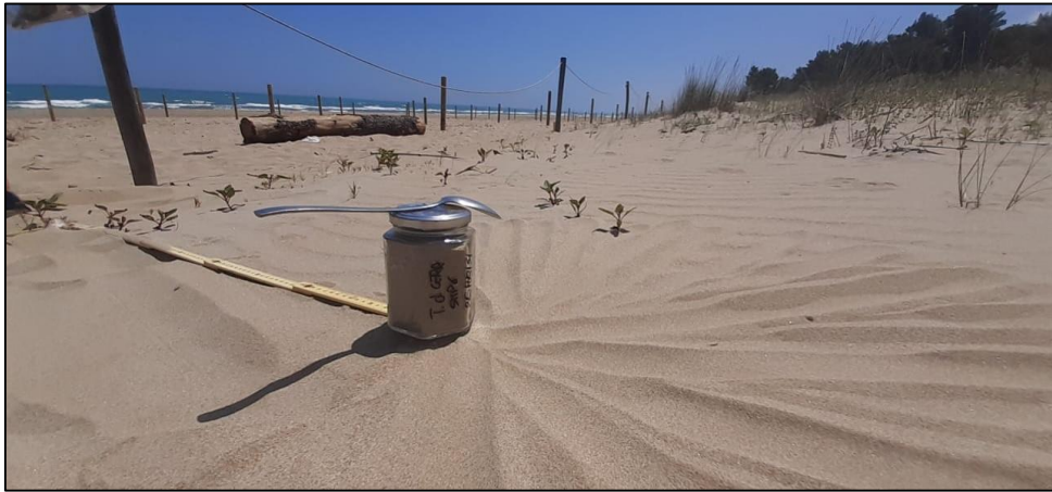
Figure 17: Example of SMP sample collected with metal spoon on the corner of LMP-square, and stored in a glass jar.
