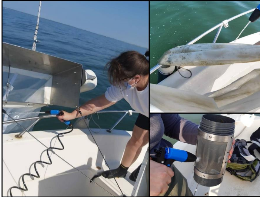
Figure 21: Manta-net has hoisted on the vessel and carefully rinsed with sea water, using a high-pressure pump.
