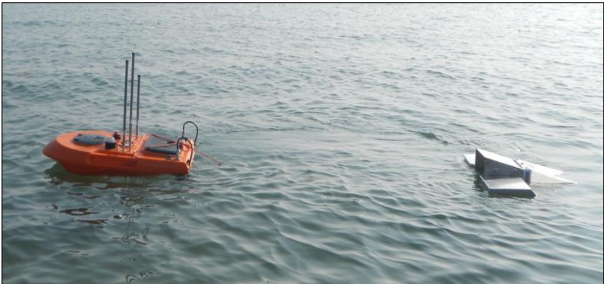
Figure 26: Integrated system (marine drone + holo sensor + OBU + mini-manta).
