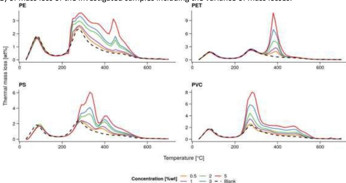
Fig. 6: Plots of TML of blank soil enriched with PE, PET, PVC, and PS, respectively, at different concentrations. (David et al., 2019)
