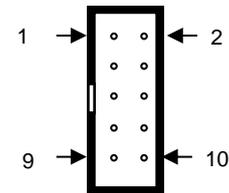
To use the serial console port, you need to open the metal case of Matrix-518 and the CON1 connector is near the reset button and LEDs. Use any terminal software such as hyper terminal and configure the setting as follow:
