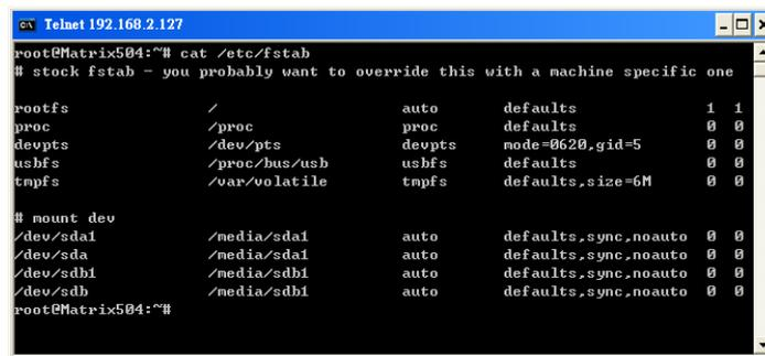
A screenshot of a Telnet window titled 'Telnet 192.168.2.127'. The window shows a root prompt at 'root@Matrix504:~#' and the command 'cat /etc/fstab' has been executed. The output displays the contents of the /etc/fstab file, which includes entries for rootfs, proc, devpts, usbfs, tmpfs, and several mount entries for /dev/sda1, /dev/sdb1, and /dev/sdb. The window has standard window controls (minimize, maximize, close) in the top right corner.
