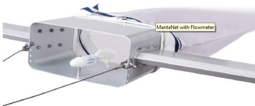
Fig.4.2 - Manta Net with volumetric sensor
