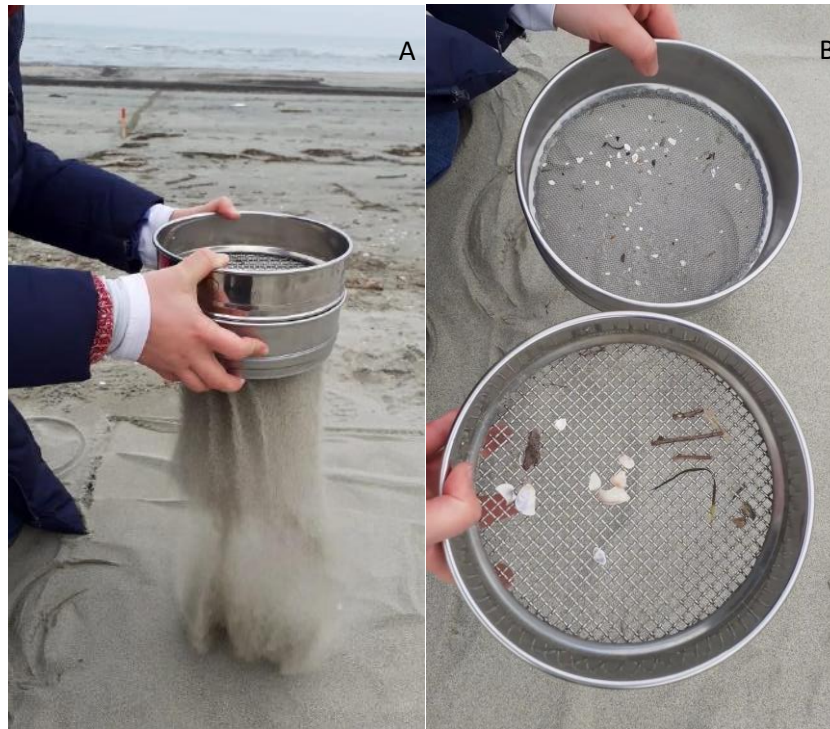
Fig. 3: A) Sieving sediments B) Material retained on the 5 and 1 mm sieves
