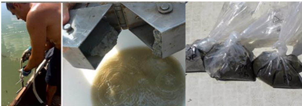
Fig. 12: Sampling with Van Veen grab
