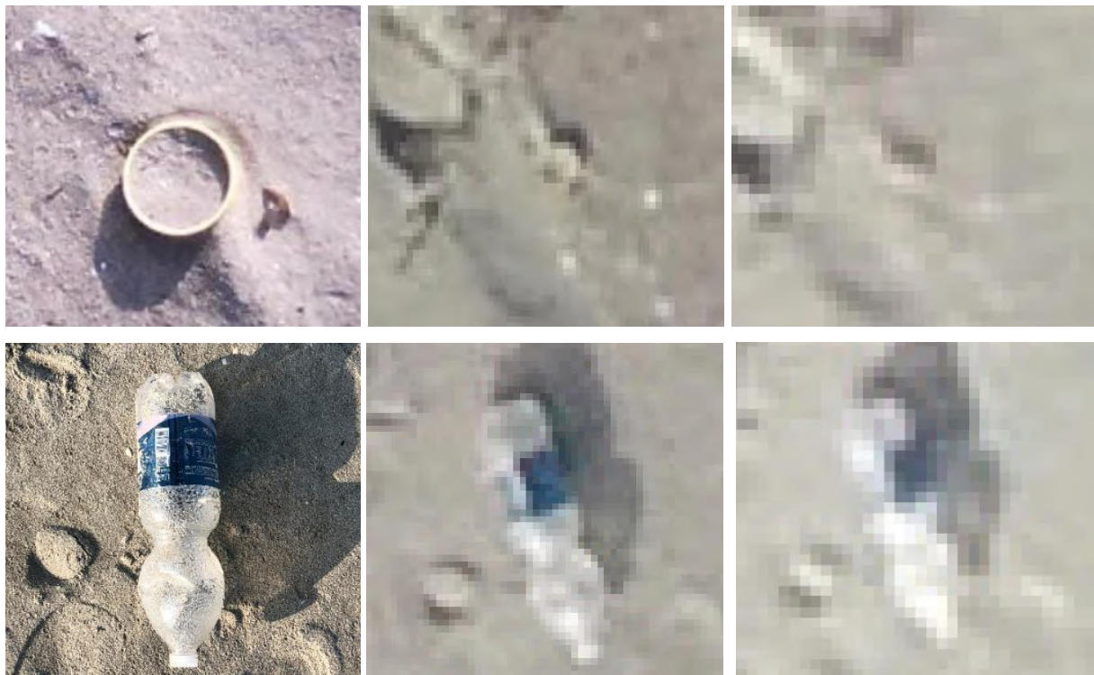
Fig. 10: From the left to the right: ground survey picture; low-altitude aerial image; high-altitude aerial image.
