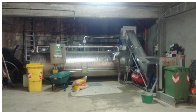
Figure 1 Electromechanical composter and auxiliary equipment set up in Fossalto
