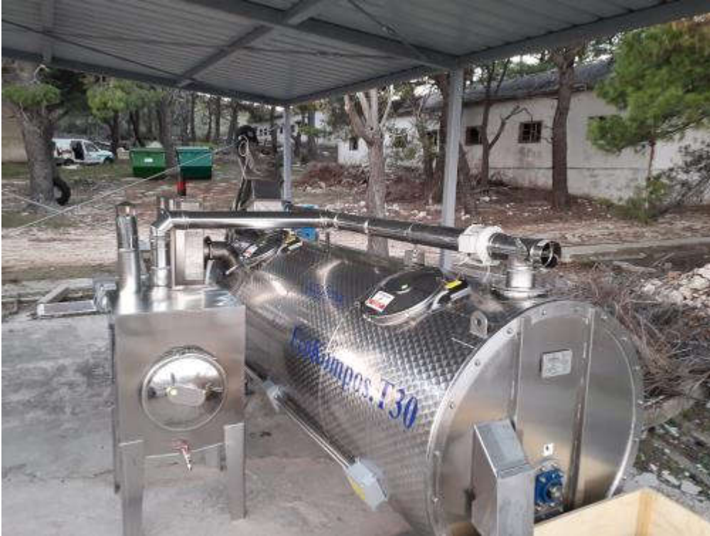
Figure 3. – The electromechanical composter installed under a roof in Ist Island
