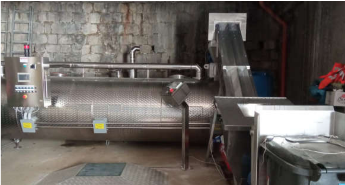
Figure 5. The electromechanical composter installed inside the municipal garage of Fossalto
