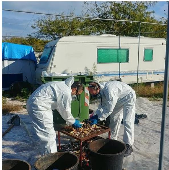
**Figure 3. –screening of the Mixed municipal waste sample withdrawn from the waste container**
