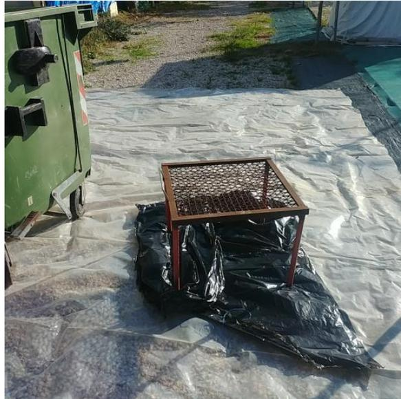
**Figure 2. – Removing fragments with a size lower than 20 mm**
